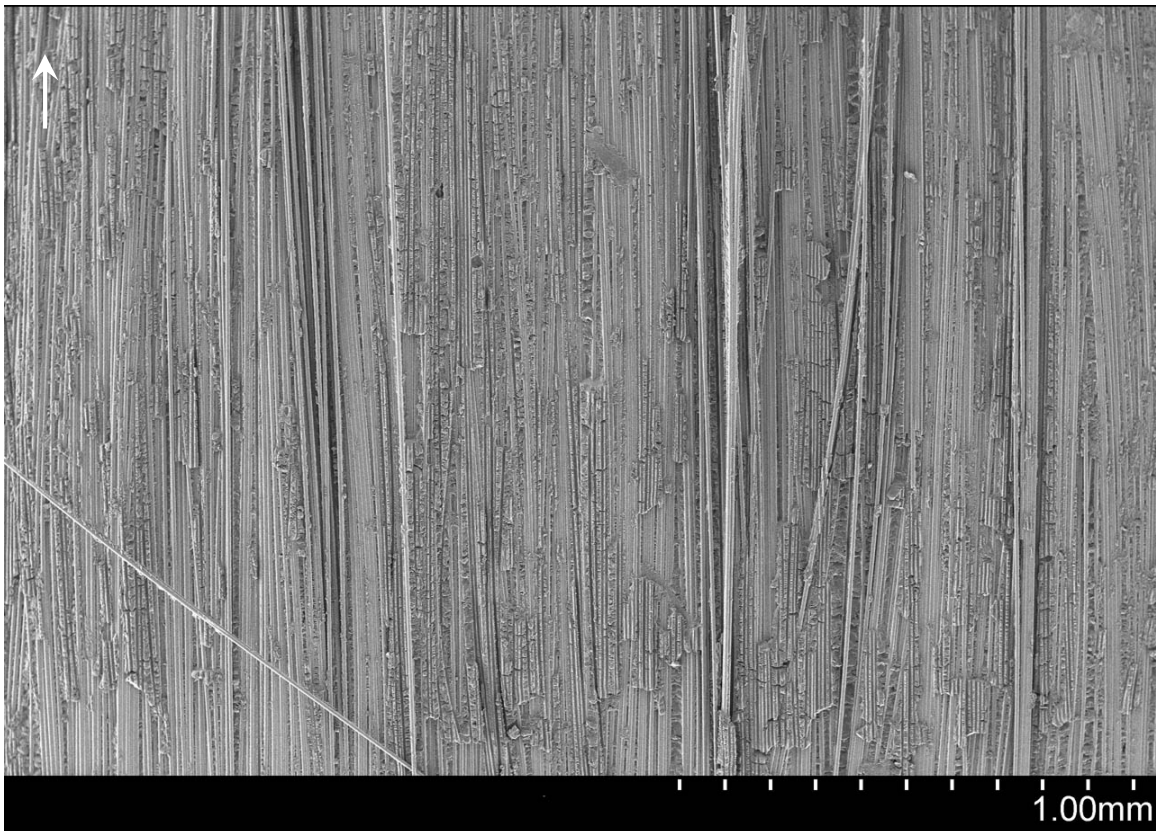
Figure 3.35: Overall view of Material B tested under Mode II loading revealing a small amount of fiber bridging, but a relatively smooth fracture surface (arrow indicates crack direction).
