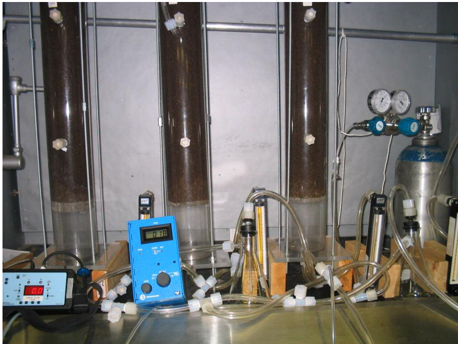
Figure 3.1 Experimental Setup with Compost
