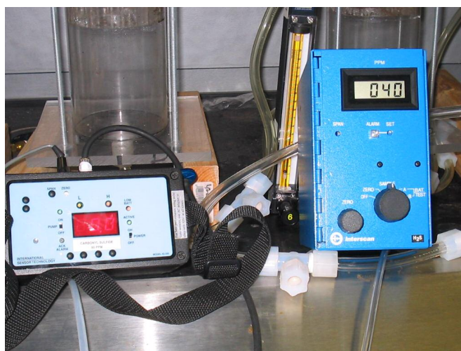
Figure 3.6 COS and H 2 S Sensors
