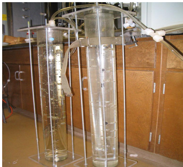
Figure 3.4 COS and H 2 S Humidification Chambers
