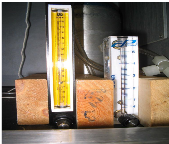
Figure 3.3 Flow Meter to Measure Gaseous Mixture (left) Air Flow Meter (right)
