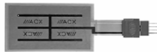
Figure 1.10 Pictures of the commercially available low-profile commercial flexible piezoelectric transducers. Most commonly, MacroFiber composites (MFCs) operating in d_{31} mode are utilized. MFCs have been extensively modeled and characterized for performance. Life-time testing on MFC's shows no changes in output power up to 1.4 million cycles.
