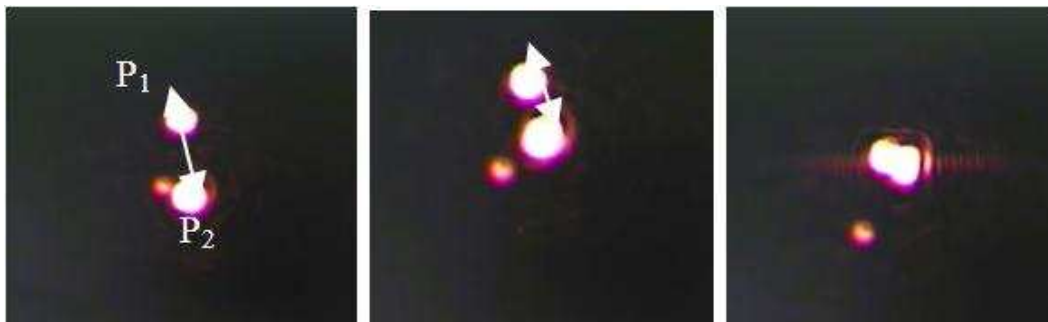
Figure 5.26. Image consisting of two laser spots projected onto a microscope CCD camera with a 5x zoom lens. Fine rotations of the beamsplitter cause the distance d between the spots to converge to zero.
