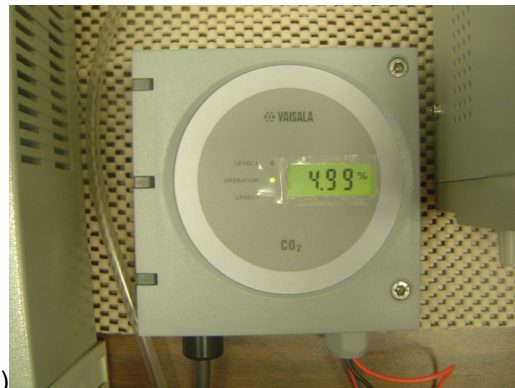
Figure 4.3: A) Image showing the aerial view of the incubator showing its parts inside along with a microfluidic device mounted inside in it with neuronal culture. B) Image showing the temperature reading inside the incubator with the set value as 35.0°C and the value being 35.2°C and C) Image showing the CO 2 percentage inside the chamber
