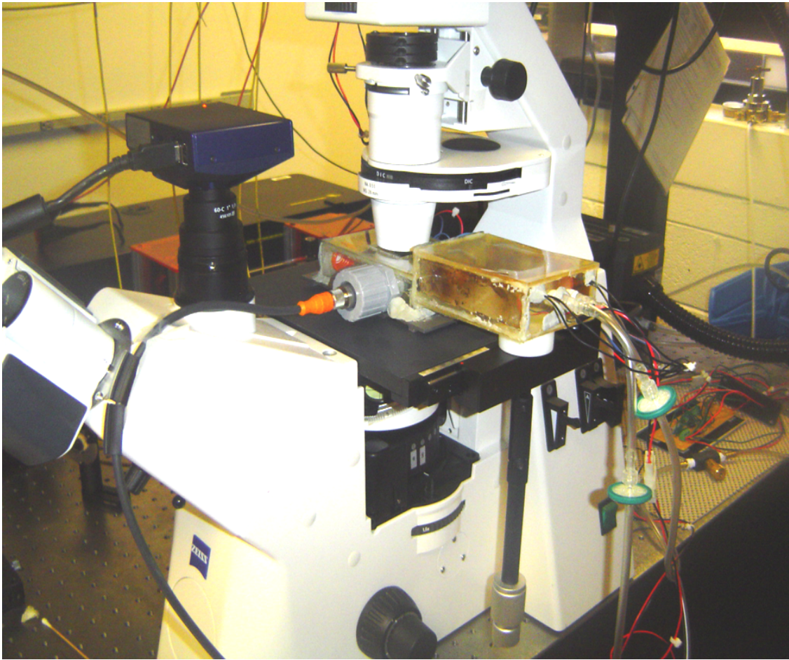
Figure 4.2: Image showing the full assembly of microscope stage incubator mounted on the microscope
