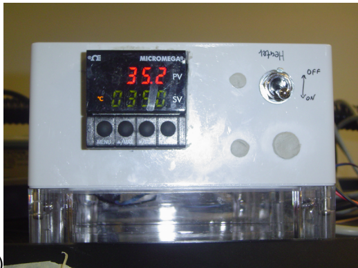
Figure 4.3: A) Image showing the aerial view of the incubator showing its parts inside along with a microfluidic device mounted inside in it with neuronal culture. B) Image showing the temperature reading inside the incubator with the set value as 35.0°C and the value being 35.2°C and C) Image showing the CO 2 percentage inside the chamber
