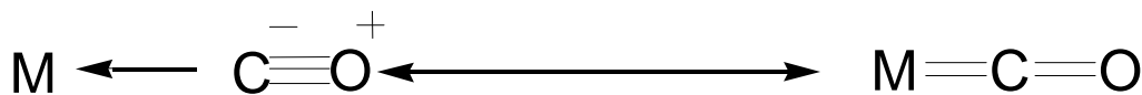
Figure 1.4. Resonance forms for coordinated carbon monoxide; left, form 1, “non-classical carbonyl, right, form 2, “classical” carbonyl
