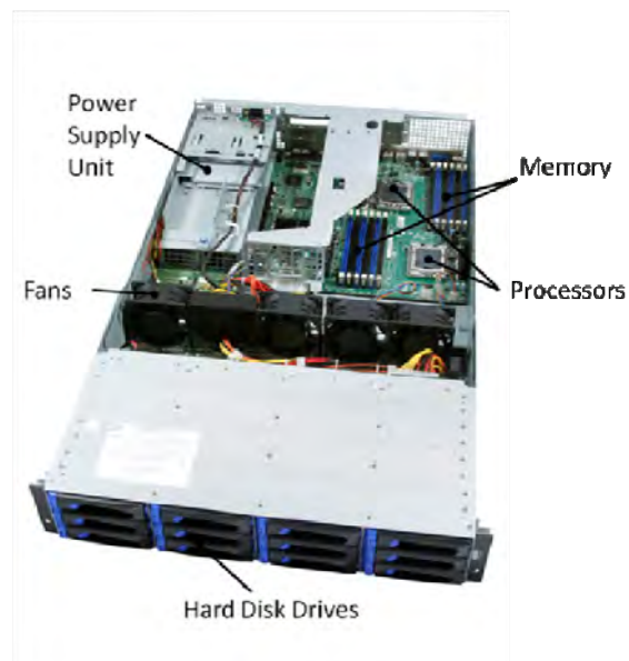
Figure 4.2 Typical Server Components [118].
