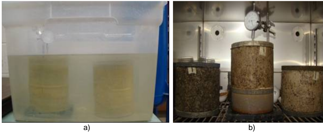
Figure 3.6 Test set up for Wetting/Drying Process a) Wetting b) Drying
