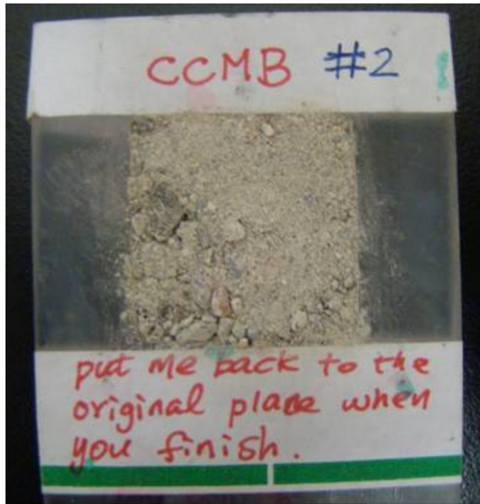
Figure 3.12 Sample holder with powdered RAP mix
