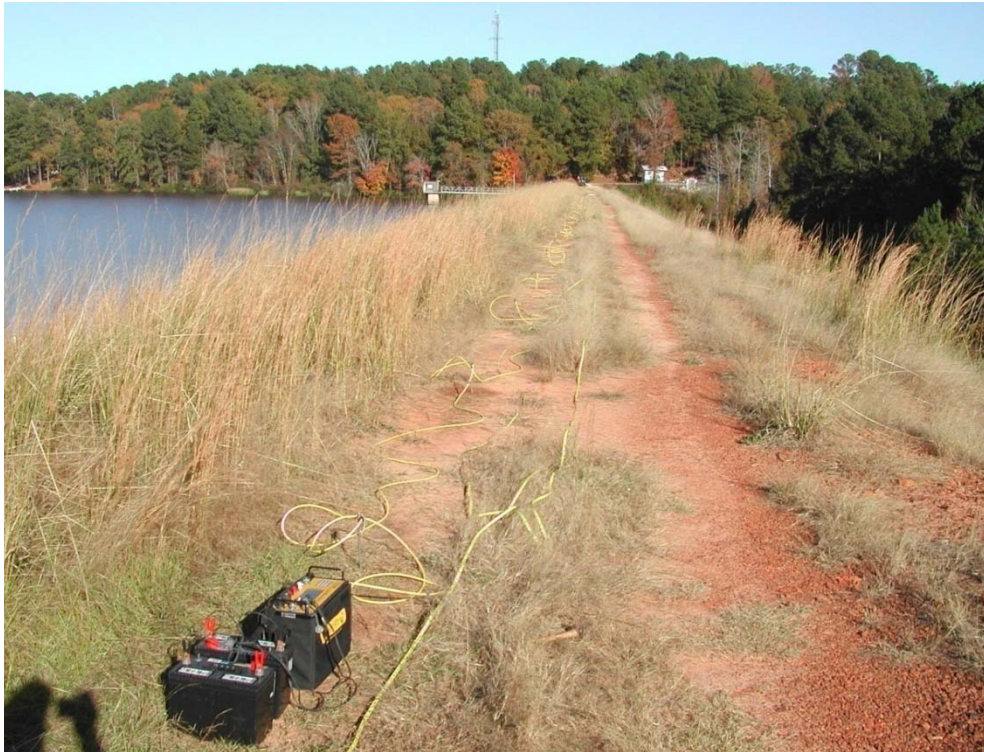
Figure 3.5 Performance of Electrical Resistivity Tomography Survey at Lake Gladewater
