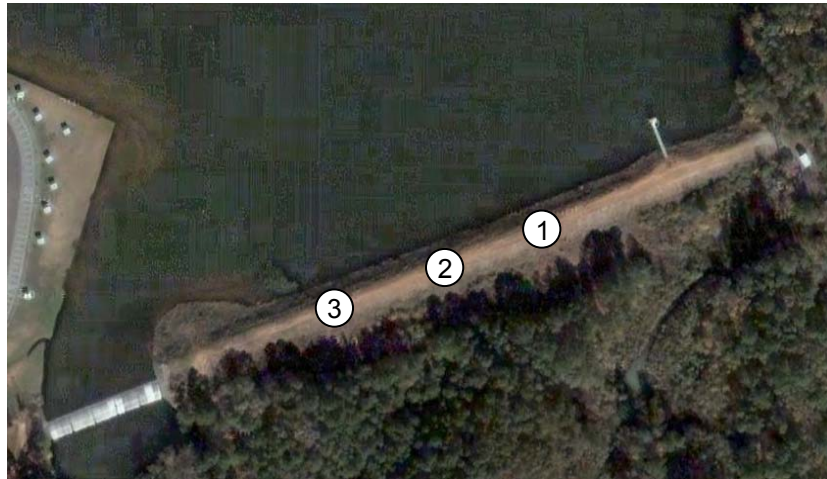
Figure 3.2 Approximate Boring Locations along Crest of Dam
