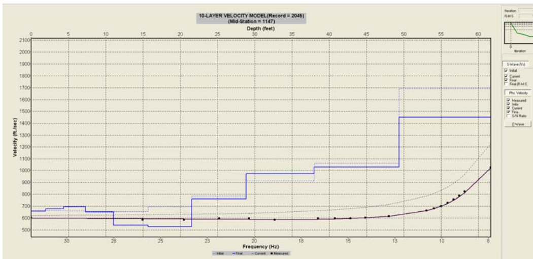
Figure 3.10 Inversion of Sounding No. 45 from Lake Gladewater Dam
