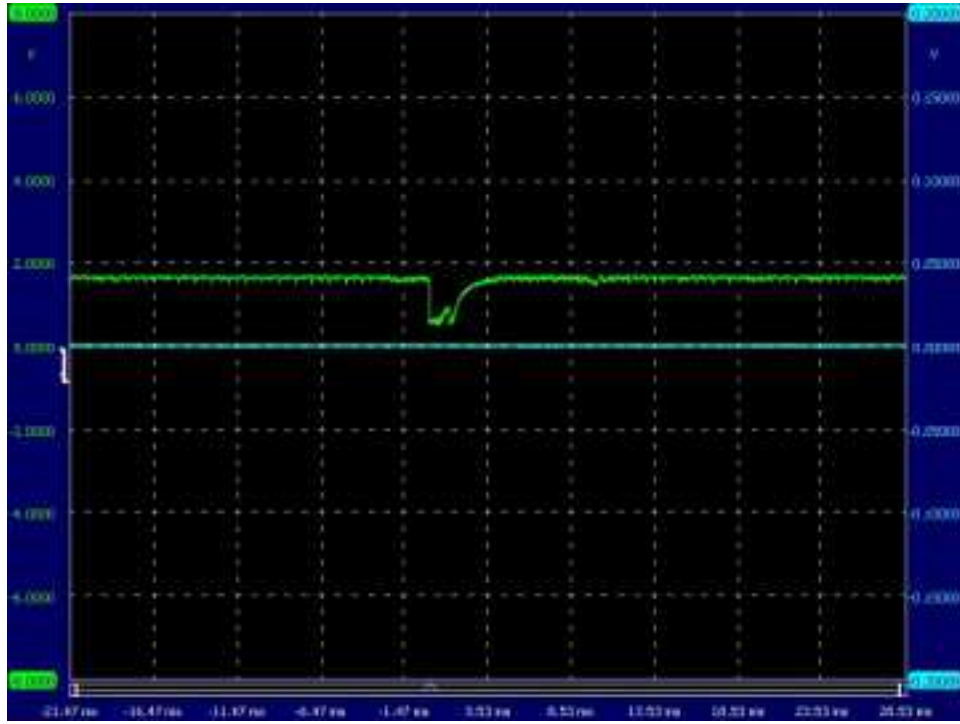
Figure 2.6. Filtered, amplified inverted output of the second stage amplifier.
