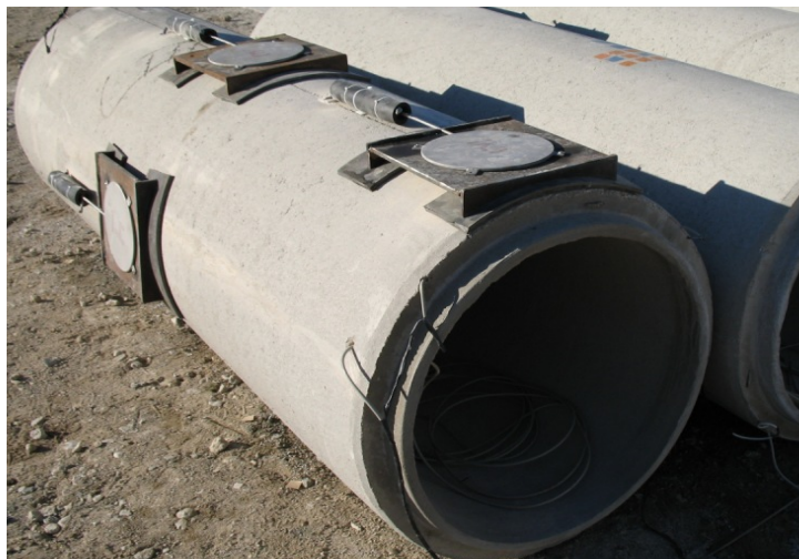
Figure 2.5 Typical test setup details for pipeline system; (a) plan view, (b) section A – A, (c) Pipe# 1 with earth pressure cells.
