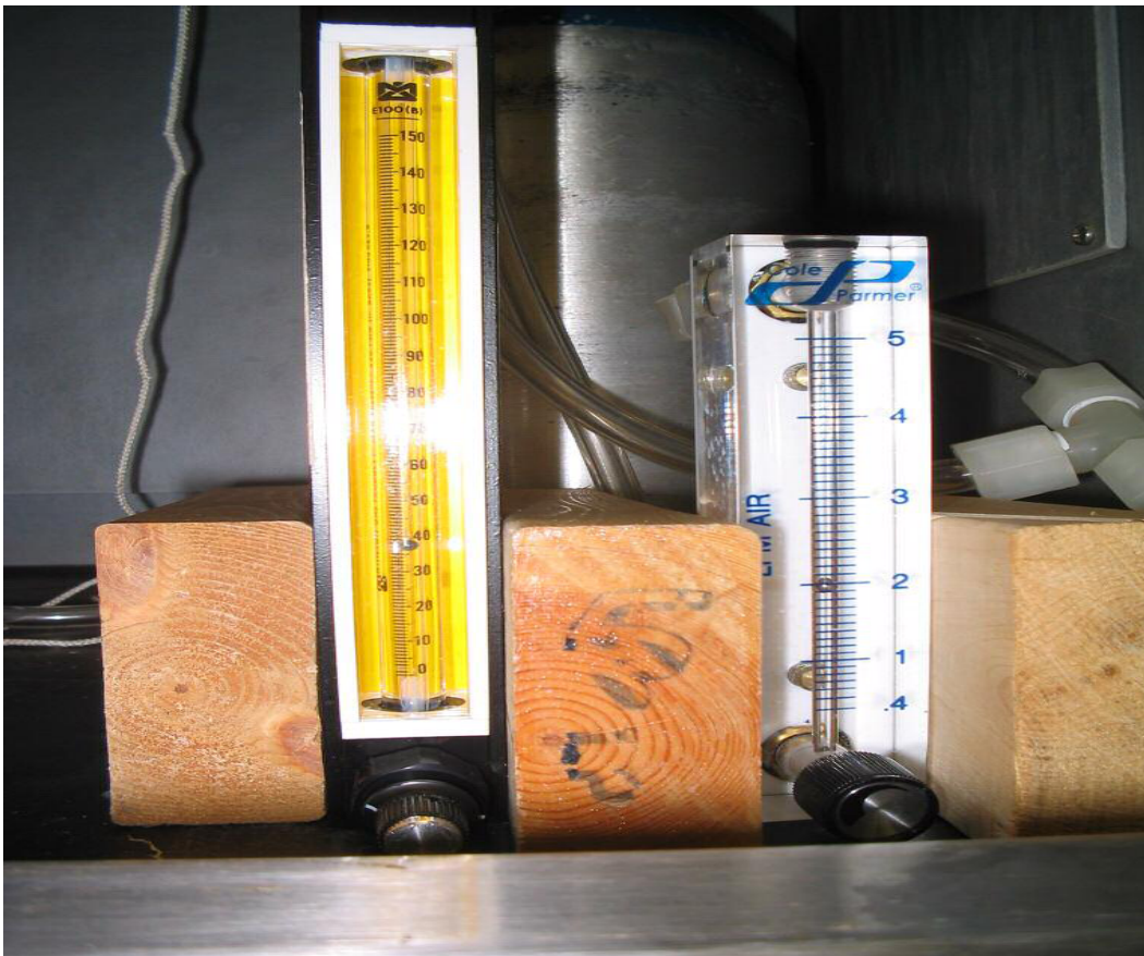
Figure 3.9 Flow Meters to Measure Gas Flow and Air Flow
