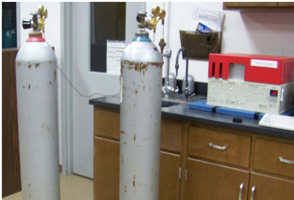
Figure 3.14 Carrier and Support Gases Attached to the Gas Chromatograph
