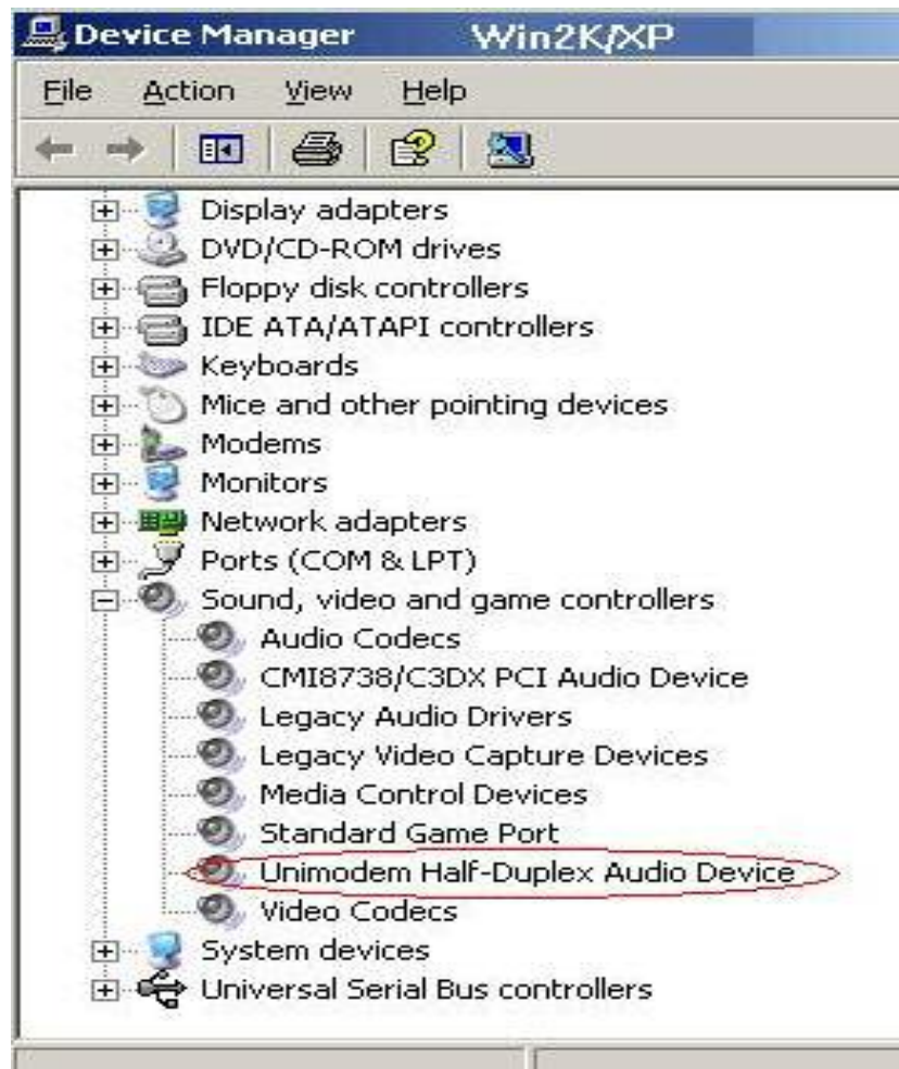
Figure 5.5 Half-Duplex Audio Device in Win XP Device Manager
