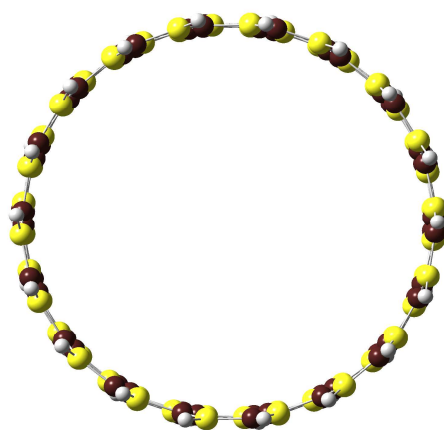
Type 3 SiCNT (9, 9) Tube diameter = 15.648 Å Radial buckling = 0.0025 Å
