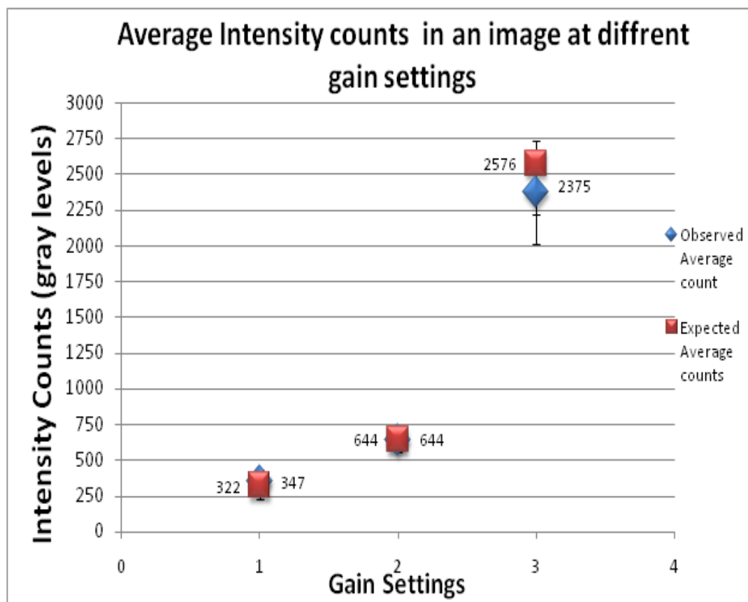
Figure 3.3 Figure shows the average intensity counts (gray levels) in each image at 3 different gain settings, gain1 is high signal to noise ratio mode with relative gain of \sim 1/2 X , gain2 is high dynamic range mode with relative gain of \sim 1X and gain3 is high sensitivity mode with relative gain of \sim 4 X . Accordingly the average intensity counts vary by a factor of 1/2 X for gain1, 1 X for gain 2 and 4 X for gain3
