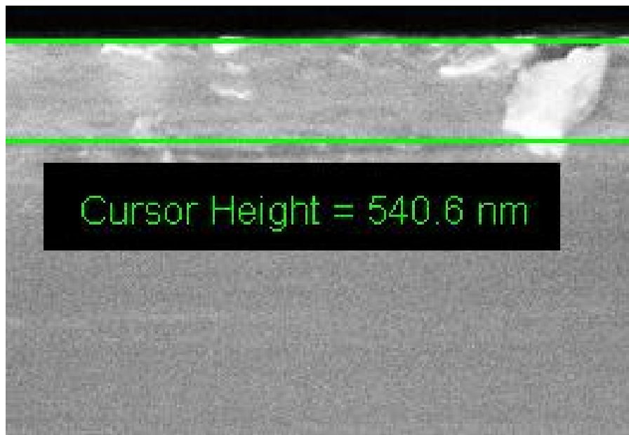
Figure 3.19 The thickness 540.6 nm after SOG spin coating.
