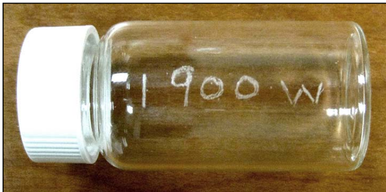
Figure 5.5 Glass vial etched with sample year and side of Prometheus. In this vial, the year was 1900 and the side was W.
