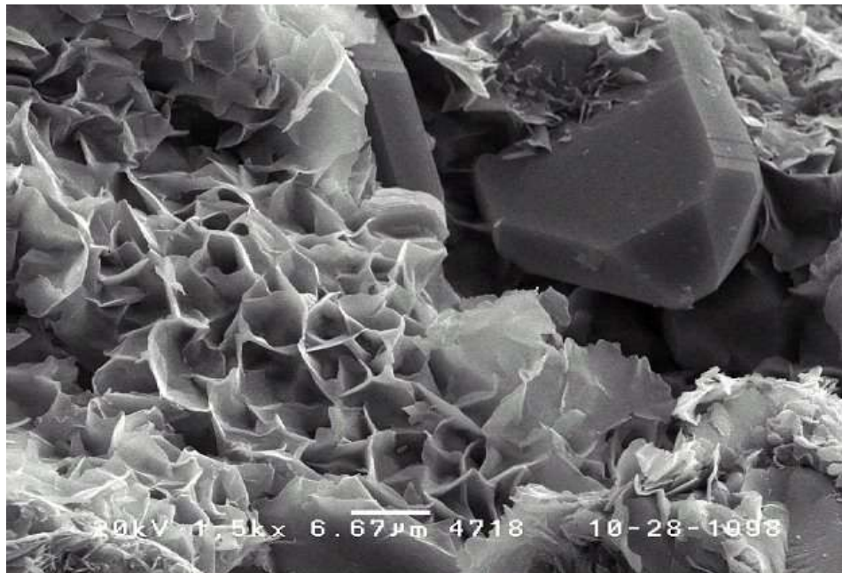
Figure 2.9 Authigenic Smectite (Montmorillonite) Overgrown on Pore Spaces and Authigenically-Overgrown Quartz Grains in Sandstone, SEM Image of a Core Sample: Scale 67 micron (OMNI Laboratories, Inc).
