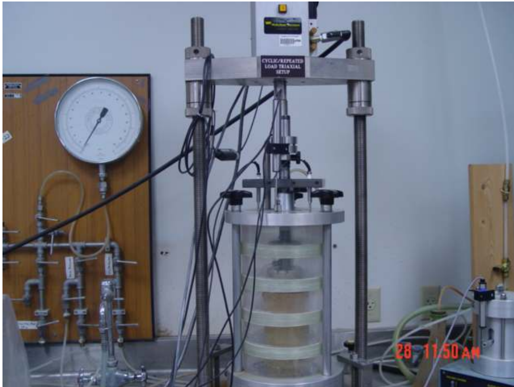
Figure 3.7 Loading frame and triaxial cell setup.
