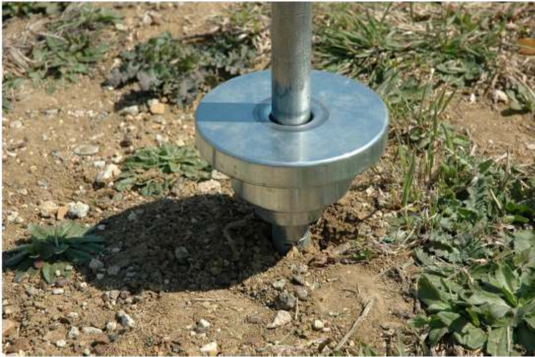
Figure 6.17 Penetrations of DCP Apparatus into the Pavement Courses.
