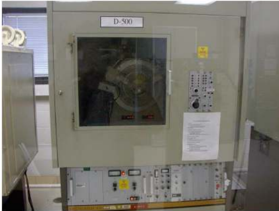
Figure 3.4 Illustration of X-Ray Diffraction Test Setup.
