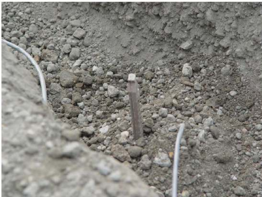
Figure 5.7 Placement of Strain Gauges (Pillappa, 2005).
