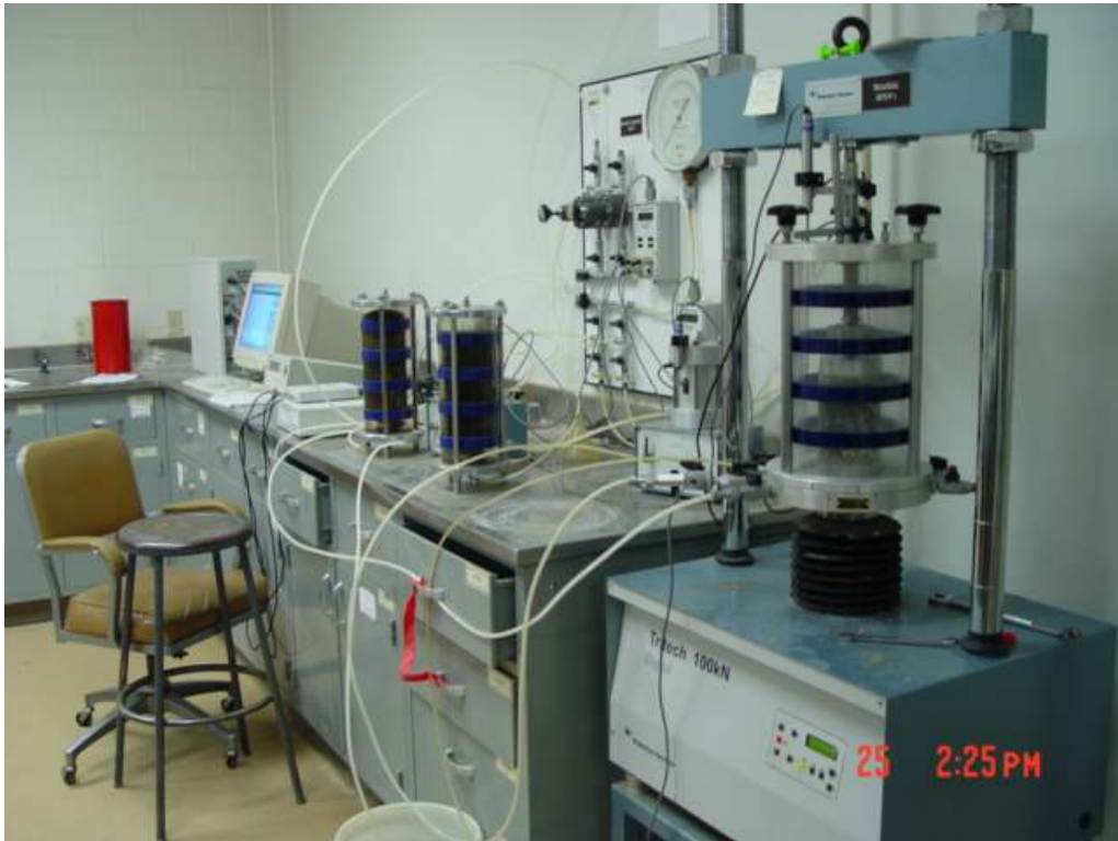
Figure 3.5 UCS Test Setup in the Laboratory.
