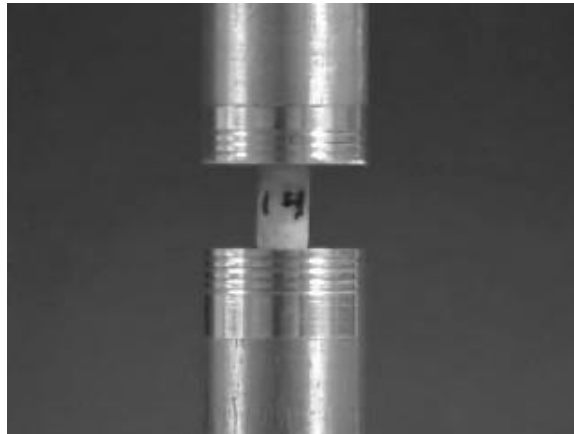
Figure 4.11 POC-HA 120-1 Specimen Compressed to 20% Strain
