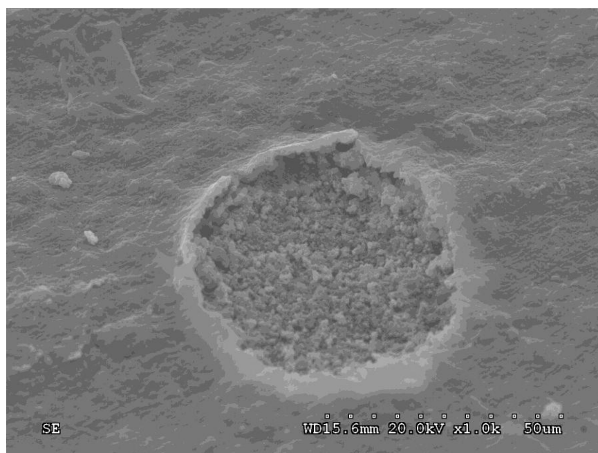
Figure 3.1 Ablated Surface with 10 Pulses at 220 mW (scale bar 50 microns)
