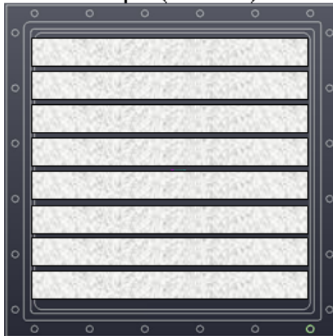
Figure 6.9 Wick Configuration having 1/2 Inch Strips (8 each)
