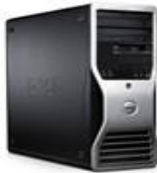
Figure 2.12 The Figure shows the Dell T3400 Workstation system. This system was chosen as it can accommodate all the PCI cards required to control the nanopatterning system. However, the installation of DMD video cards in the system reduced the rate of image display.
