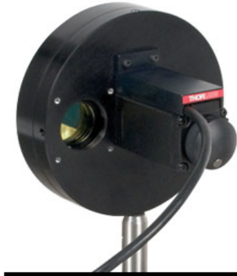
Figure 2.10 The figure shows the FW103S Filter wheel. The 340 and 380nm filters are installed on it. The movement of the filter positions is controlled by a controller which is in turn controlled by an APT that is called as a sub-routine from NI LabView.
