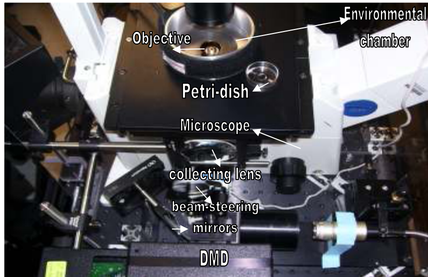
Figure 2.3 The figure shows the DMD with the microscope and the integrating optics. The DMD is connected to the CPU via a set of video cards that transmit the gray scale pattern to the DMD. The Petri-dish, objective, beam-steering mirrors and collecting lens are also indicated to depict the light path from DMD to the Petri-dish.
