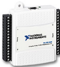
Figure 2.11 The Figure depicts the NI-USB 6008 that was used as the Digital control board to provide TTL pulses to the strobe lamp and the SenSys Photometrics camera. [60].
