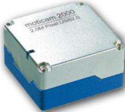
Figure 2.7 The Figure depicts the Motic CCD camera used on the system. The USB camera is used to locate the channels in a given specimen.
