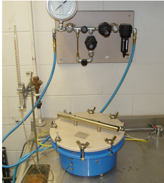
Figure 3.10 Closed pressure vessel after applying air pressure
