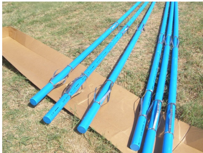
Figure 4.32 Assembled inclinometer casings of 4.5 m (15 ft) long
