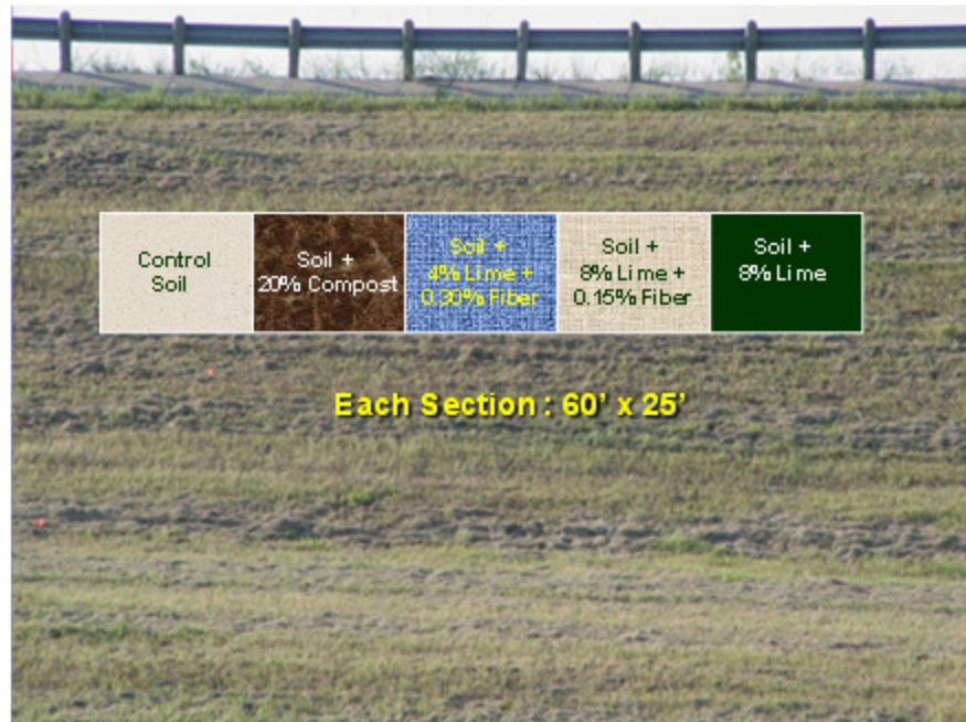
Figure 4.4 Layout for construction of test section 18 m x 7.5 m (60 ft x 25 ft)
