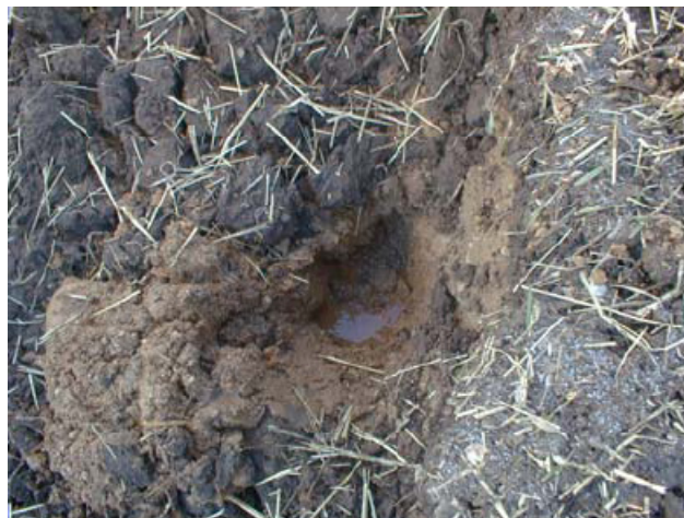
Figure 2.39 Perched water on a failure surface through seepage (Source: Titi and Helwany, 2007)
