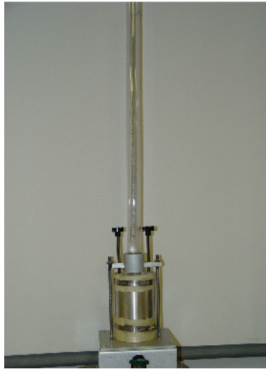
3.13 Setup of permeability test
