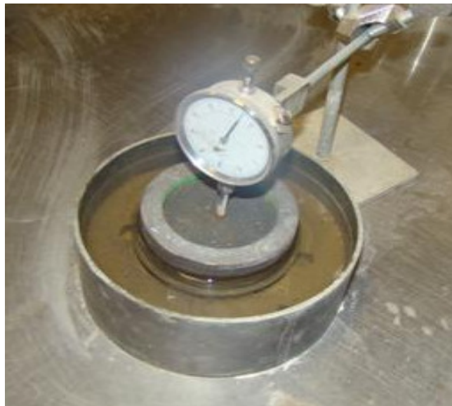
Figure 6.16 Test set up for vertical swell strain test
