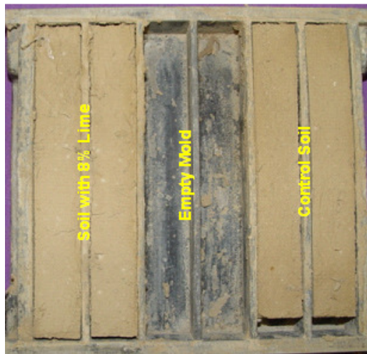
Figure 3.2 Linear shrinkage test setup
