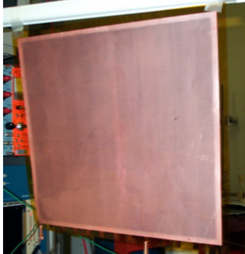
Figure 2.1 A photograph of a large 3M-UTA GEM foil developed for 30 x 30 cm 2 prototype double GEM chambers.
