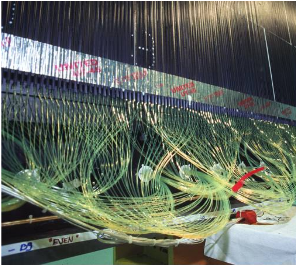
Figure 1.11 The fiber double readout system going into the PMT's.
