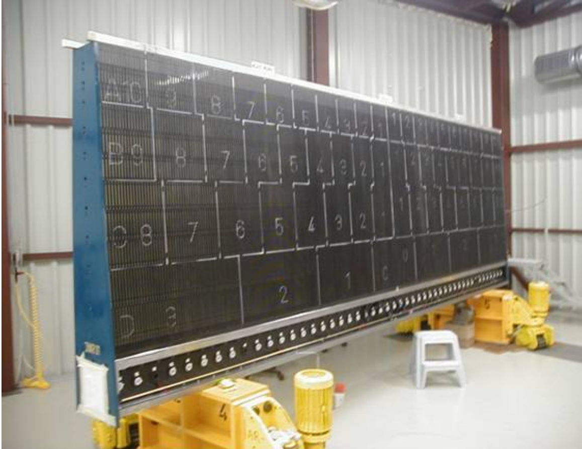
Figure 1.12 The cell segmentation of a Long barrel module before placing the fibers.
