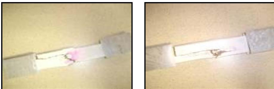
Figure 3.2 Typical Splitting Failure in Tensile Test – 6 in (152 mm) with node
