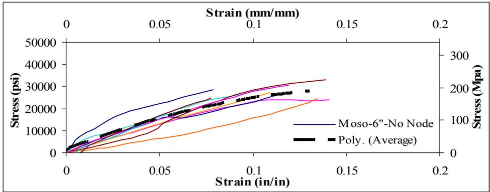
Figure 3.17 Stress-Strain Curve for samples no node
