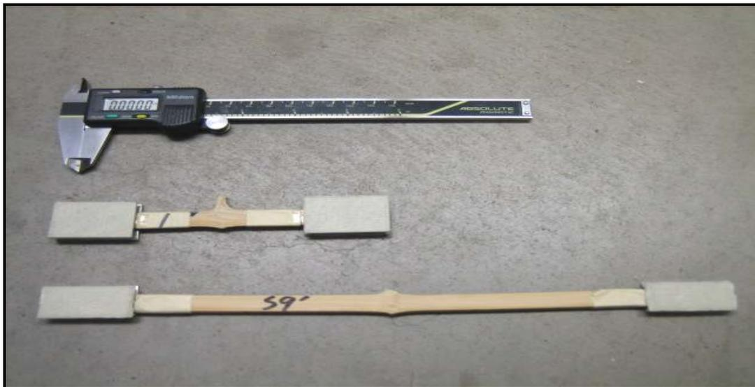
Figure 2.6 Diagram of Tensile Sample
