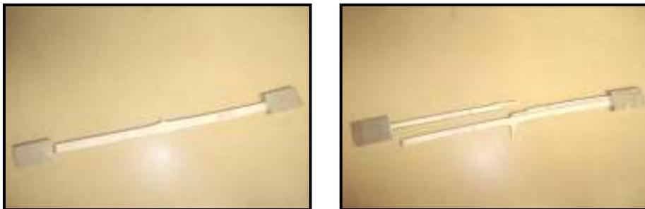
Figure 3.8 Typical Failure of the End-Tap in Tensile Test – 12 in (304 mm) with node
