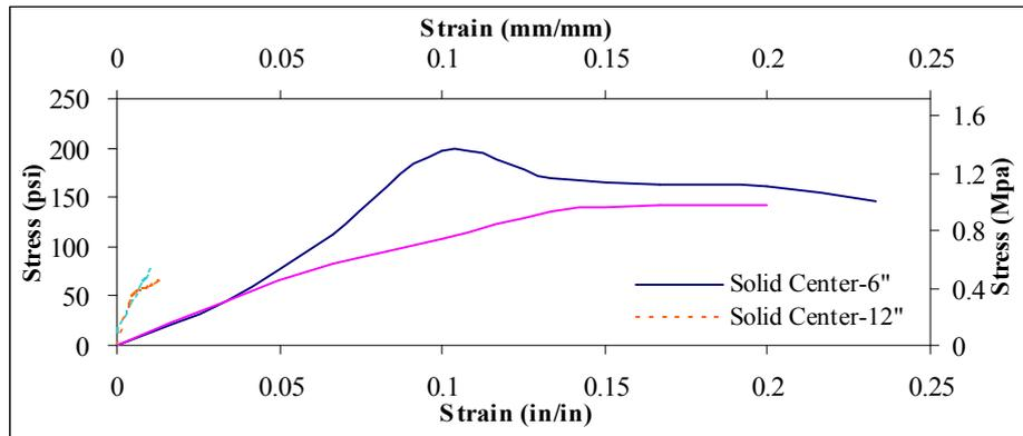
Figure 3.28 Bond Stress-Slip Behavior for Solid Bamboo - Center
