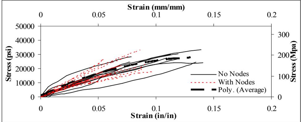
Figure 3.19 Stress-Strain Curve of Moso 6 in sample with no node & with node
