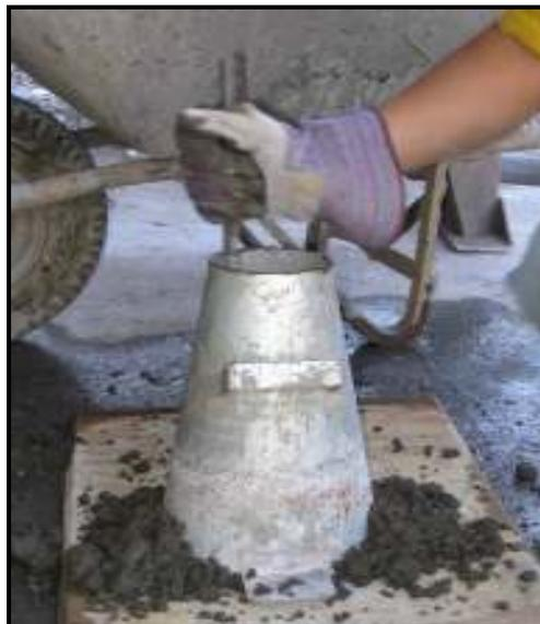
Figure 2.13 Tamping of Slump Test with Rod
