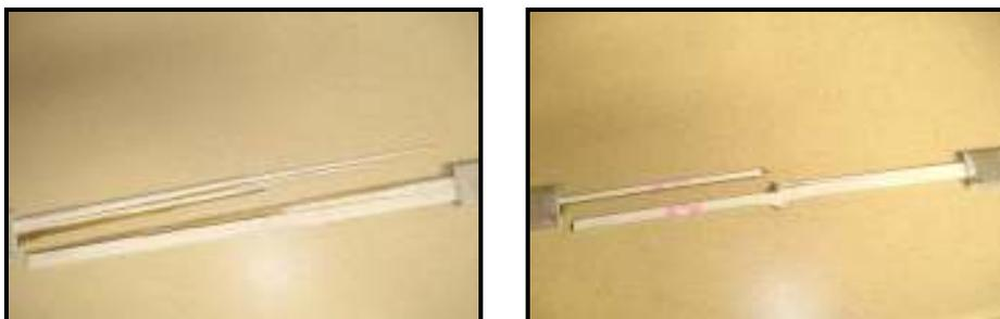
Figure 3.4 Typical Splitting Failure in Tensile Test – 12 in (304 mm) with node
