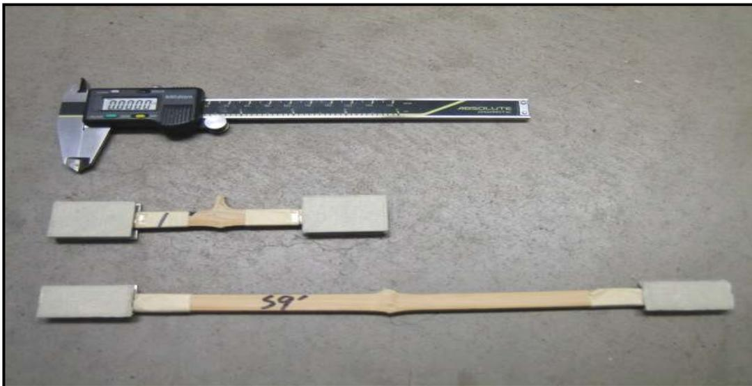
Figure 2.6 Diagram of Tensile Sample
