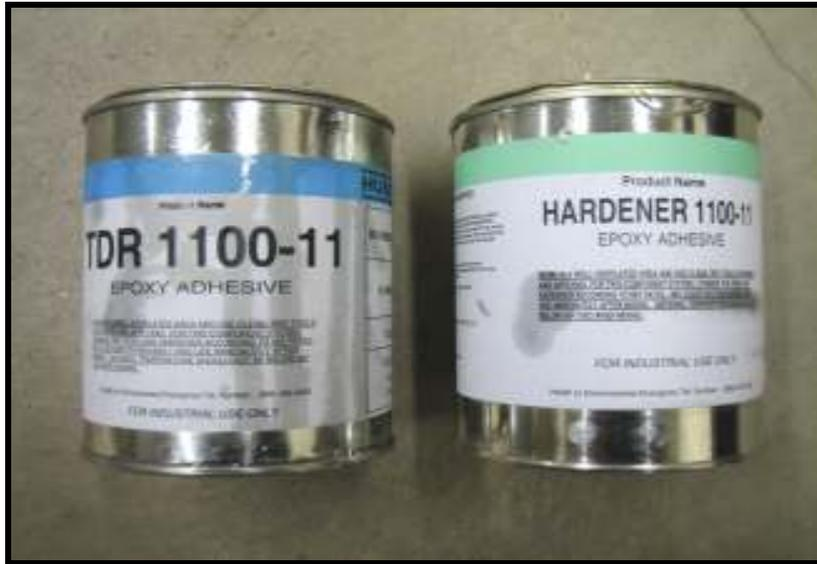
Figure 2.5 Epoxy Adhesive (TDR 1100-11 & HARDENER 1100-11)
