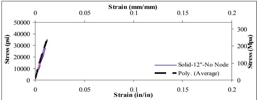
Figure 3.14 Stress-Strain Curve for samples no node
