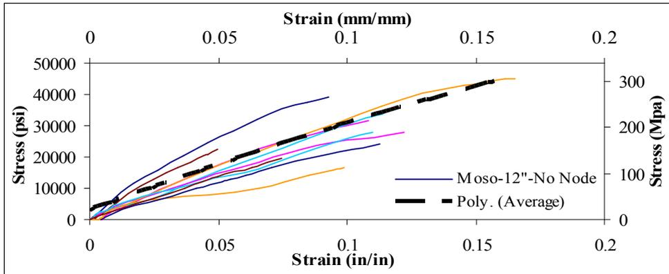
Figure 3.20 Stress-Strain Curve for samples no node
