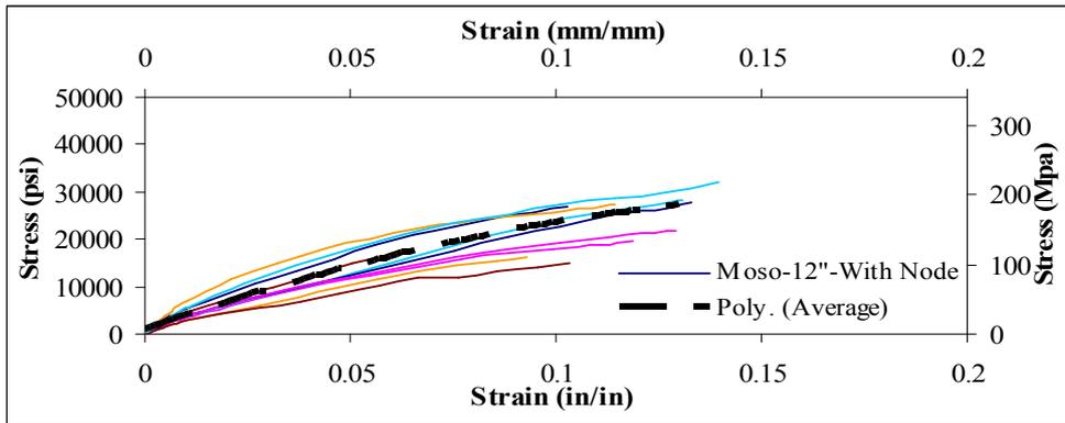
Figure 3.21 Stress-Strain Curve for samples with node
