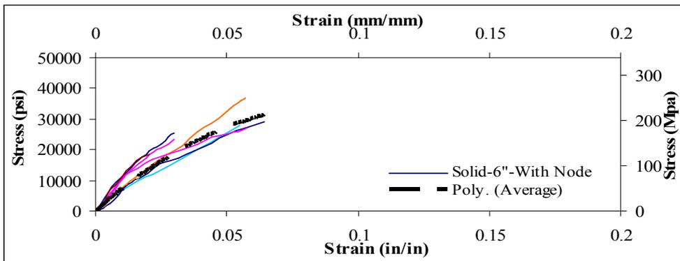
Figure 3.12 Stress-Strain Curve for samples with node
