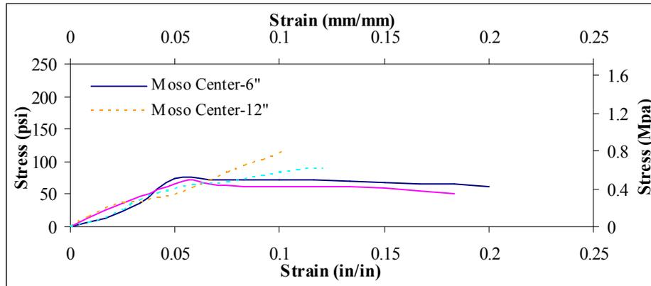
Figure 3.31 Bond Stress-Slip Behavior for Moso Bamboo - Center
