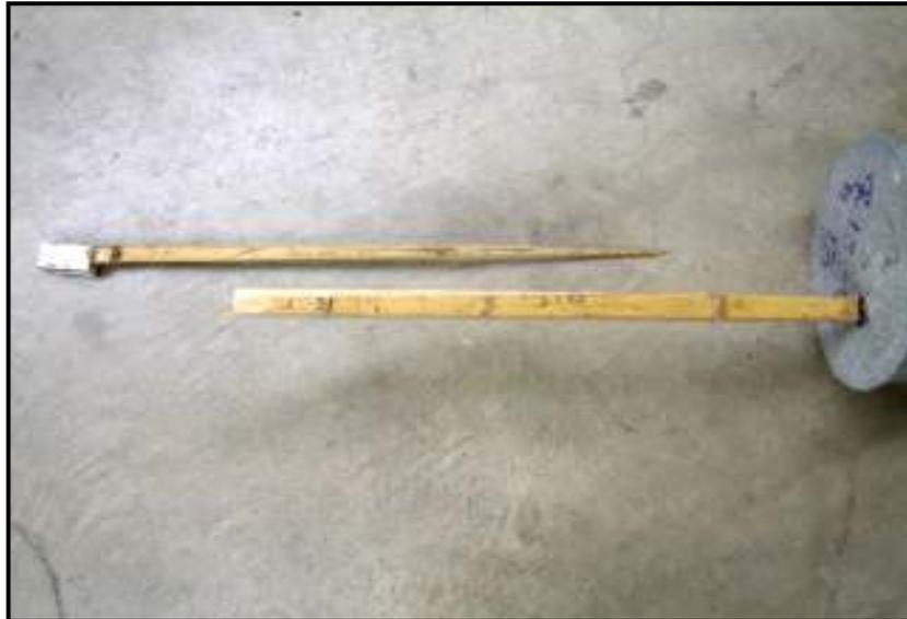
Figure 3.25 The Grip Failure of Pullout Test
