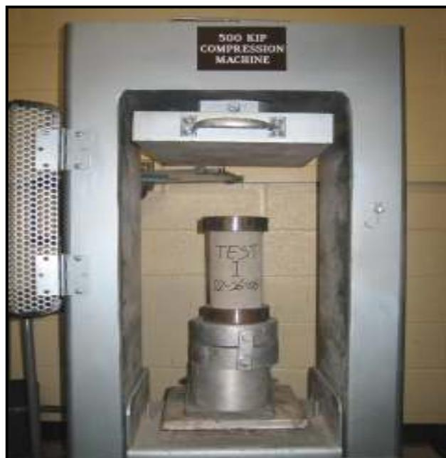
Figure 2.16 Compressive Testing
