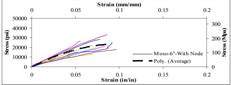
Figure 3.18 Stress-Strain Curve for samples with node
