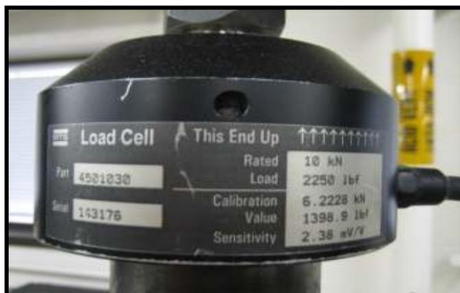
Figure 2.8 Load Cell
