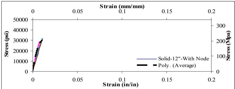
Figure 3.15 Stress-Strain Curve for samples with node
