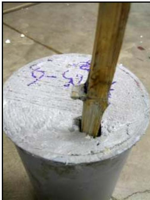
Figure 3.24 Pullout Failure Specimen
