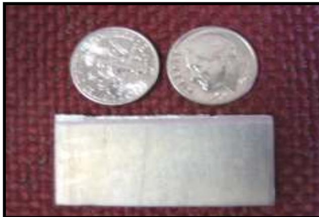
Figure 2.4 Photograph of the Aluminum Tab
