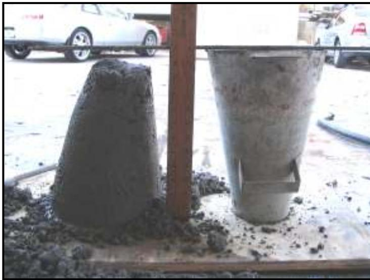
Figure 2.14 Slump Test Result
