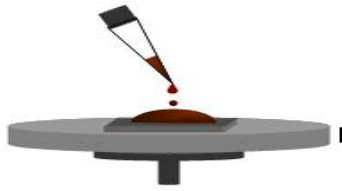
Fig. 8 Solution dispensed at the center of the substrate [46]
