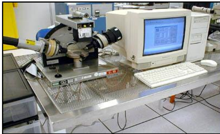
Fig. 57 Gaertner Ellipsometer for thickness measurement [69]
