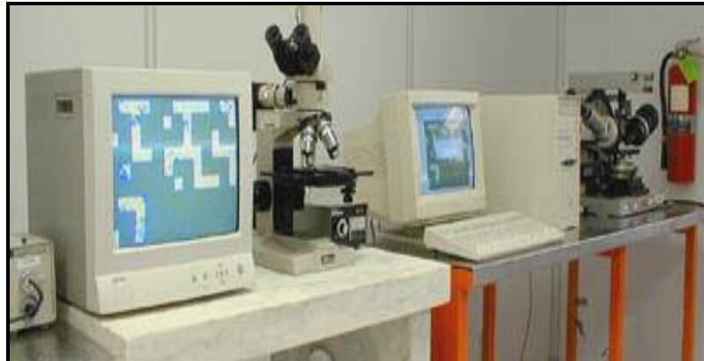
Fig. 59 Nomarski Microscope in cleanroom, UTA NanoFAB center [71]
