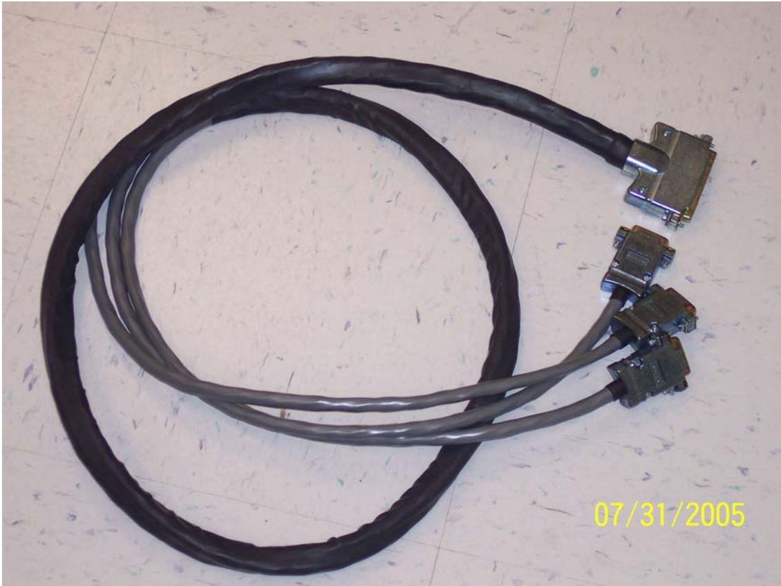
Figure 3.6. Cable interface between Newport 8016 LD/TEC controller and EDFAs.
