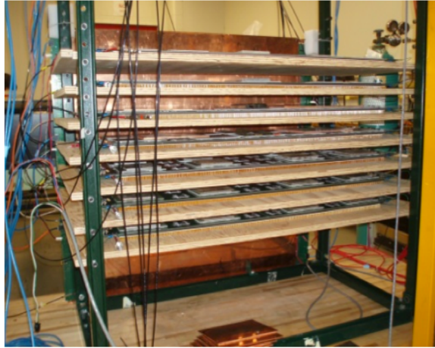
Figure 3.11. Photo of the CRTS used to validate chamber assembly and measure RPC performance.
