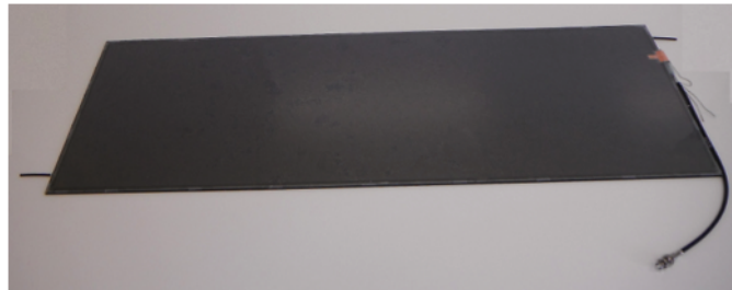
Figure 3.9. Photo of a completed RPC.
