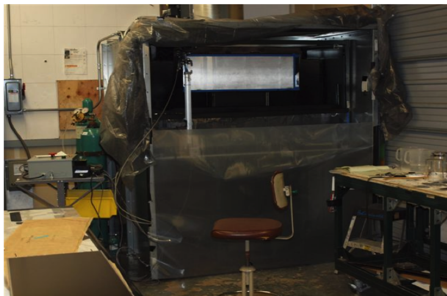
Figure 3.1. Photo of the paint booth used to apply paint to RPC chambers.
