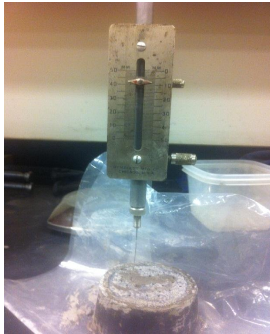
Figure 4.10: Setting time test - Penetration of needle less than 10 mm
