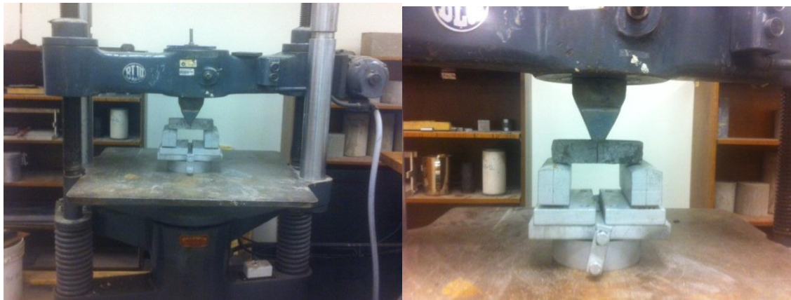
Figure 3.8: Flexural strength - (a) Loading frame for flexural strength test, (b) Center point loading setup for flexural strength test
