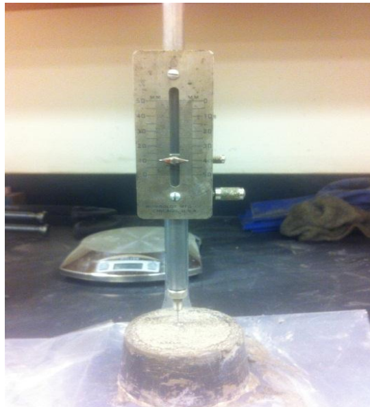
Figure 4.9: Setting time test - Vicat's needle touching the bottom of the sample
