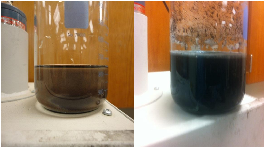
(a) (b) Figure 3.4: a and b CNT mixture before and after sonication
