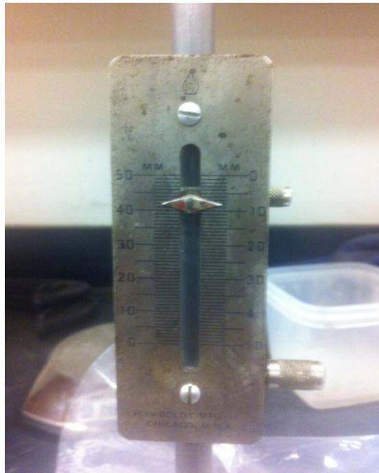
Figure 4.11: Setting time test - Reading scale of Vicat's apparatus
