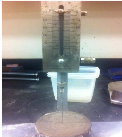
Figure 4.8: Setting time test - Vicat's needle touching the surface of mortar
