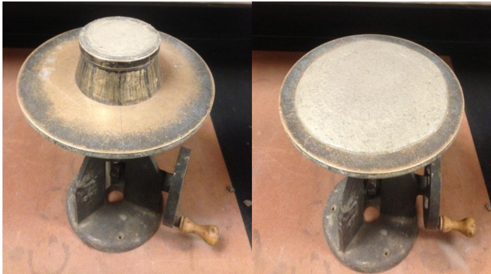
(a) (b) Figure 3.9: (a) Flow table and (b) Flow of nanocomposite after the drop
