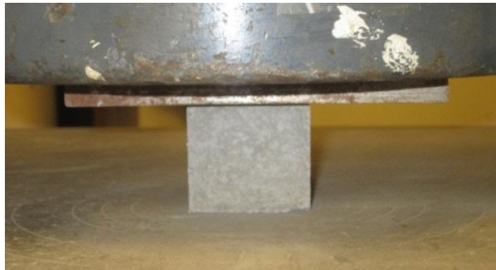
Figure 3.7: Compressive strength - 2 inch (50mm) cube under the loading plane
