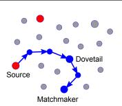
Step 2: Source constructs Egress Segment to Matchmaker via Dovetail
