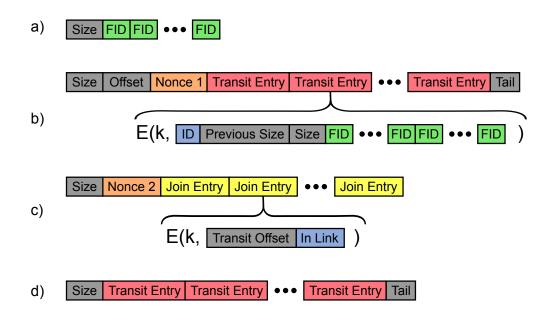
Figure 4.5. Structure for each Dovetail header segment type: a) Unencrypted header segment. b) Transit header segment. c) Join header segment. d) Approach header segment.
