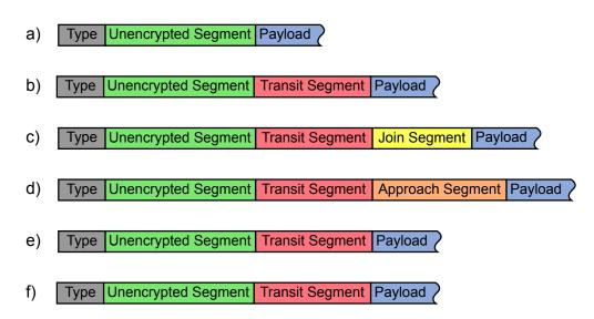
Figure 4.4. Structure for each Dovetail packet type: a) Plain packet. b) Path construction packet. c) Joinable path construction packet. d) Approach construction packet. e) Encrypted data packet. f) Encrypted response packet.
