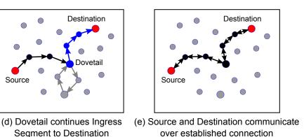
Figure 4.2. Construction of a Dovetail connection.
