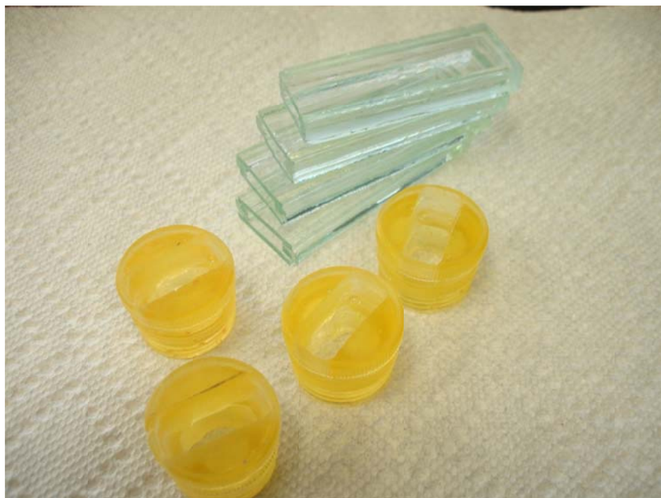
Figure 3.3 The glass reservoir and the epoxy connectors were made separately and then attached together to form the complete structure of the B type cases.
