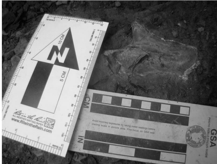
Figure 8.5 Field data collection methods; fossil mapped in situ and photographed with a north arrow and scale.
