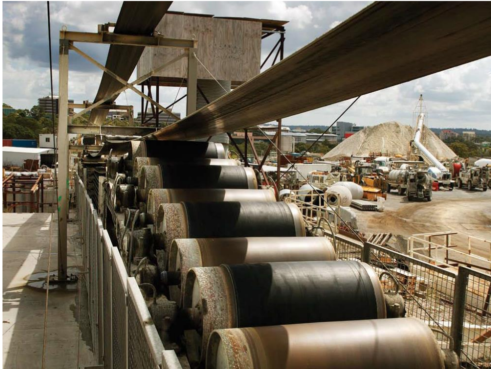
Figure 1.7. The storage cassette for a continuous conveyor system. The weaving between rollers will help to keep the belt in tension (Source: Robbins).
