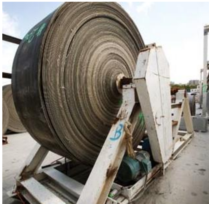
Figure 1.8. A splice stand that holds a roll of conveyor belt for a continuous conveyor
