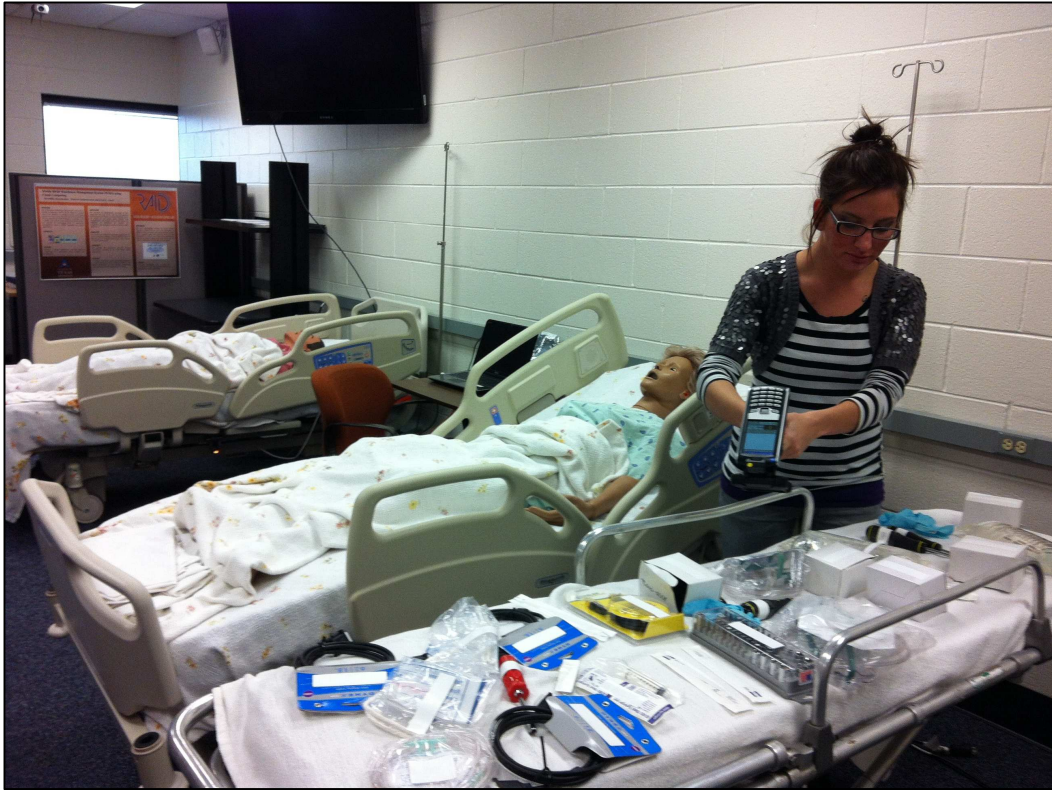
Figure 3.7: An experimenter is reading the tags by RFID handheld
