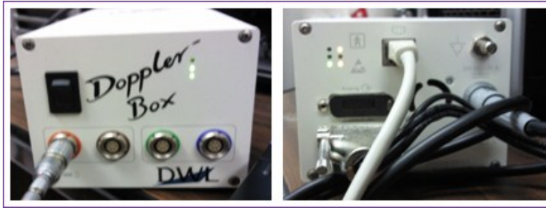
Figure 2.3 Front and Rear Panel of the Doppler-Box™
