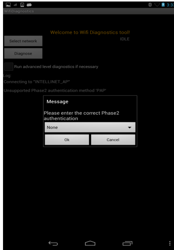
Figure 2.7 – Phase2 authentication error scenario; the user will have to set proper phase2 authentication method for the application to try reconnecting to the AP.
