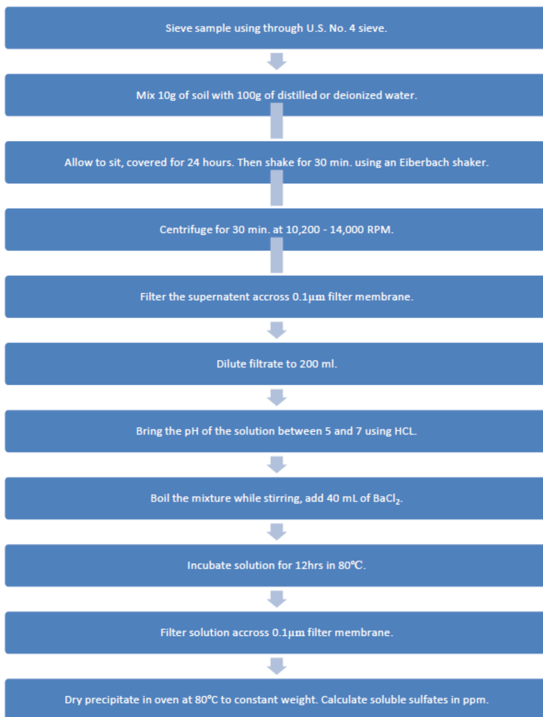
Figure 3.4 UTA Soluble Sulfate Determination for Soils Flow Chart (Puppala et al 2002)
