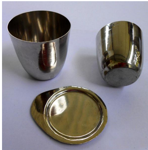
Figure 3.2 Platinum Crucible Used in AASHTO T 290 – 95 Method A (Gravimetric) Photo Source : VRS Laboratory
