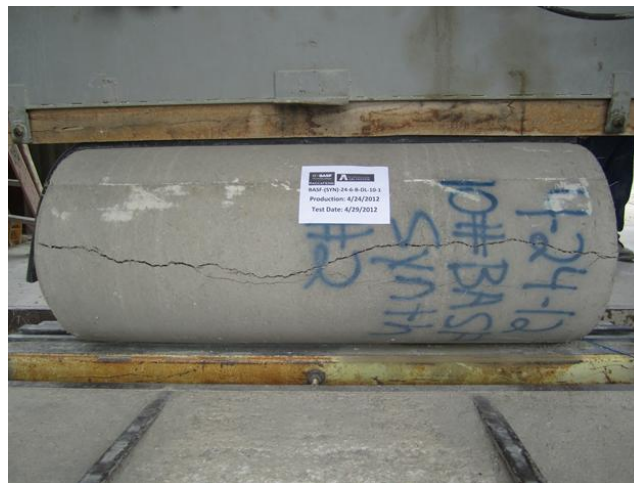
Figure E27 (b) Crack Propagation for BASF-(SYN)-24-6-B-DL-10-1
