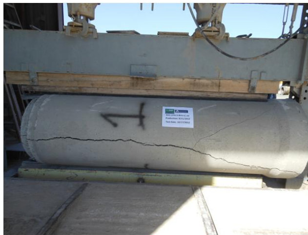
Figure E25 (b) Crack Propagation for BASF-(SYN)-24-8-B-DL-8-1-NC
