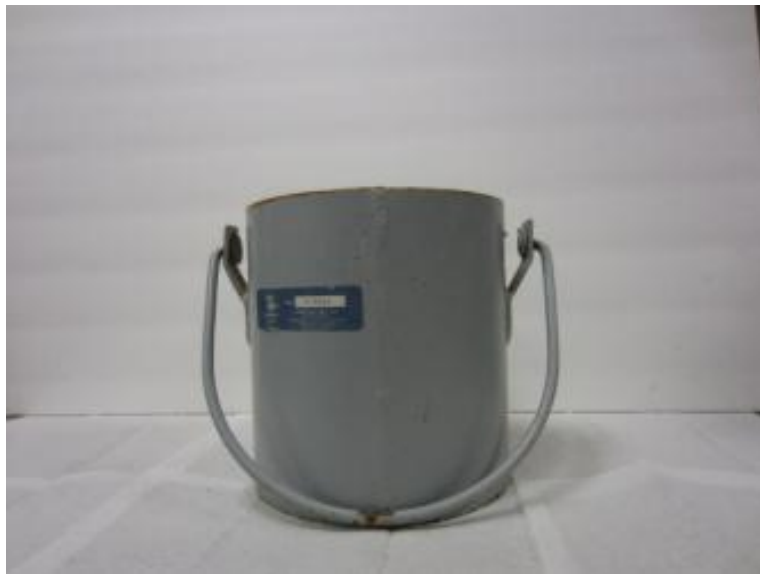
Figure 3.7. Steel measure for density measurement
