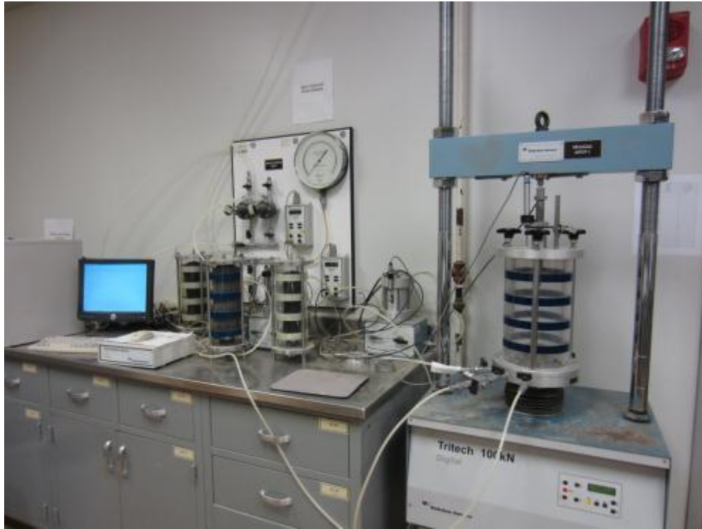
Figure 3.10 UCS test setup with Data Acquisition System
