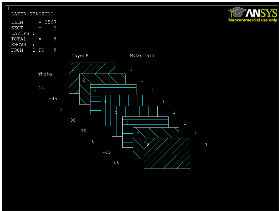
Figure 4.2 Laminated with stacking sequence of [45/-45/0/90] s
