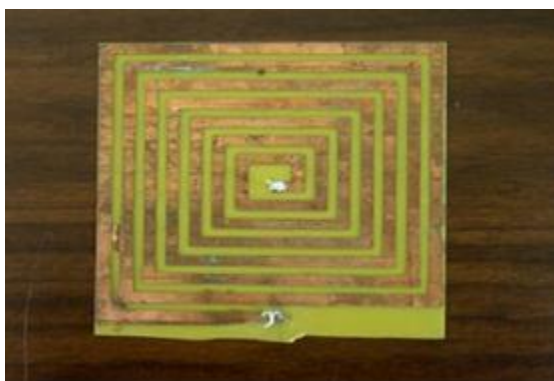
Figure 2.6 Fabricated antenna using photolithography process
