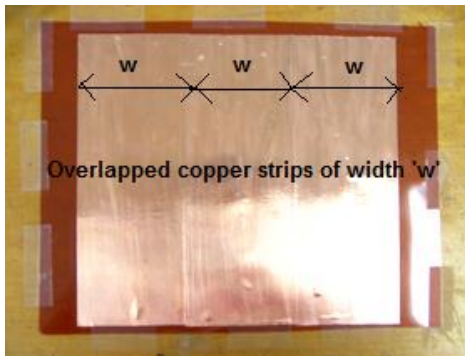
Figure 2.9 Copper strips stuck on kapton substrate
