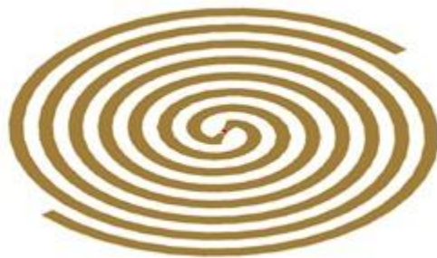
Figure 2.2 Archimedean spiral antenna [31]
