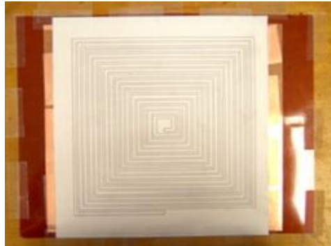
Figure 2.10 Mask taped on copper layer
