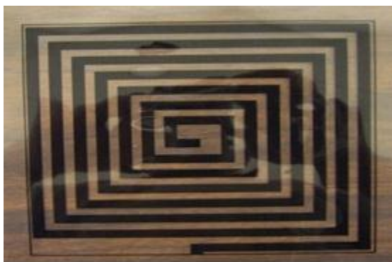
Figure 2.5 Mask for photolithography process
