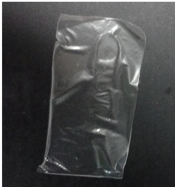
Fig. 3.1 Fabrication of elastin film. The film can be seen with some roughness and smoother surface when compared to collagen film in the Fig. 2.2.
