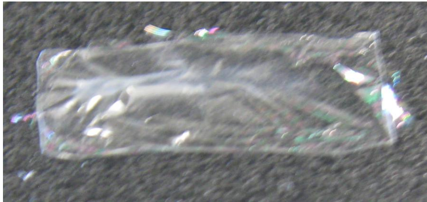
Fig. 2.2 Fabrication of collagen film.a) below shows the dried collagen film on PDMS mold after solvent casting for several hours, and b) shows the peeled film.
