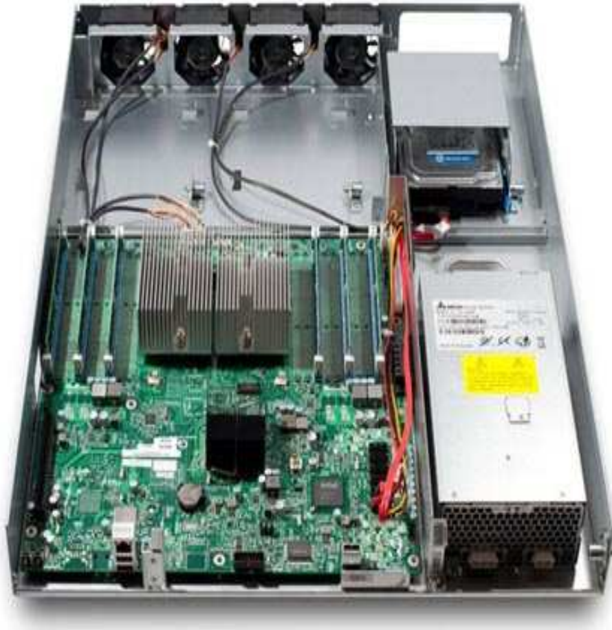
Figure 5 Open compute server [7]
