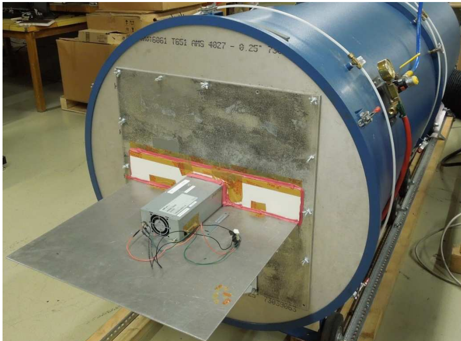
Figure 26 PSU static pressure drop measurement experimental setup
