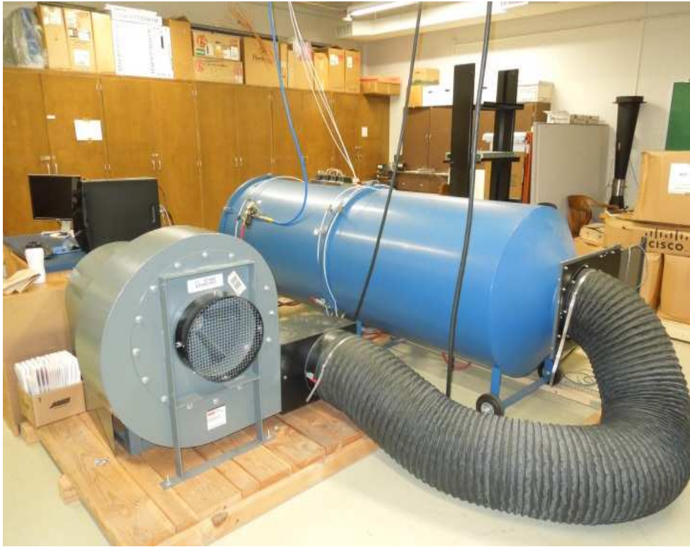
Figure 14 Airflow test bench
