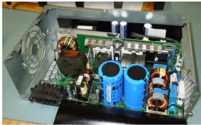
Figure 33 Power supply unit
