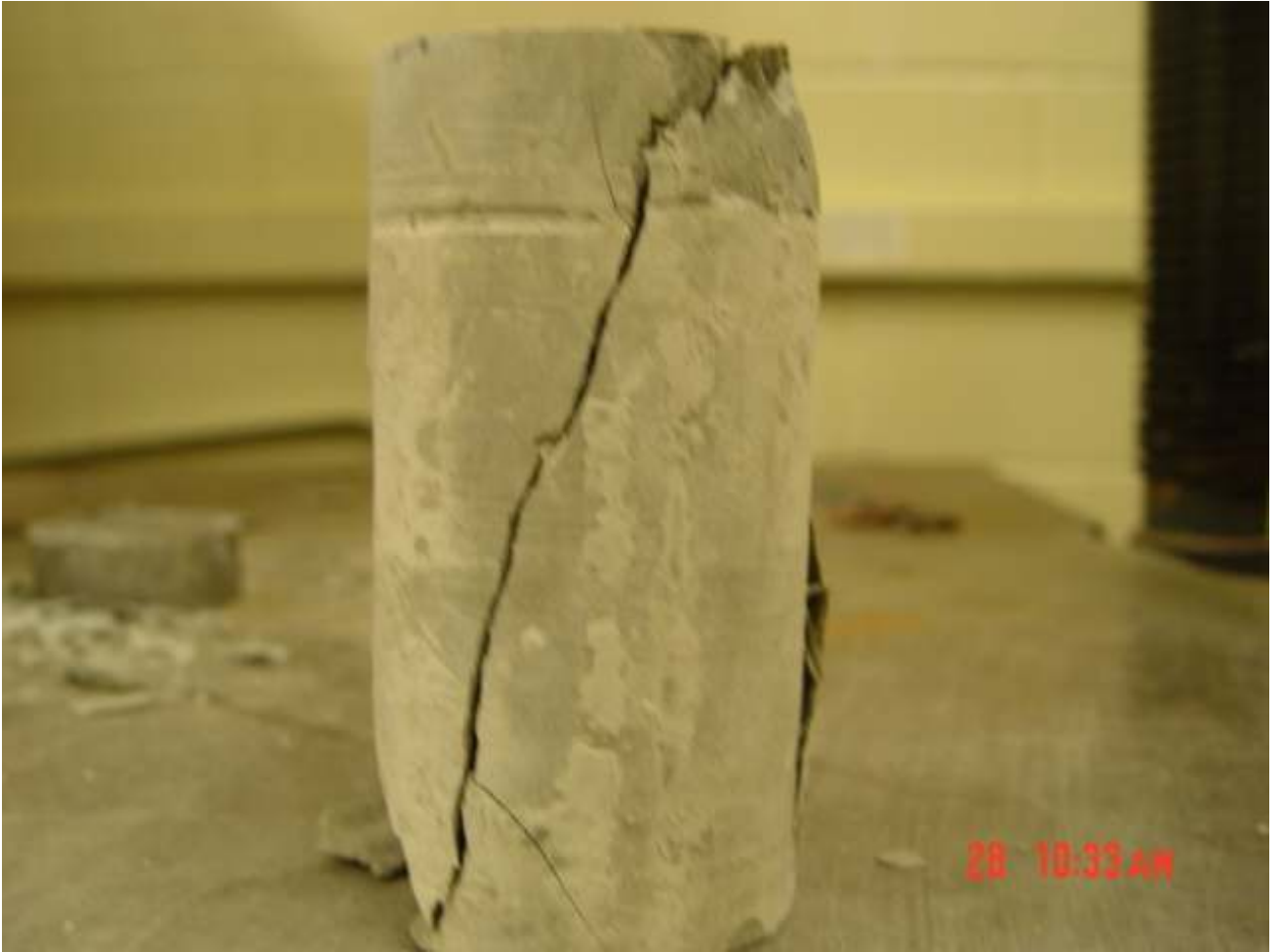
Figure A.6 Failure of Sample in an UU Triaxial
