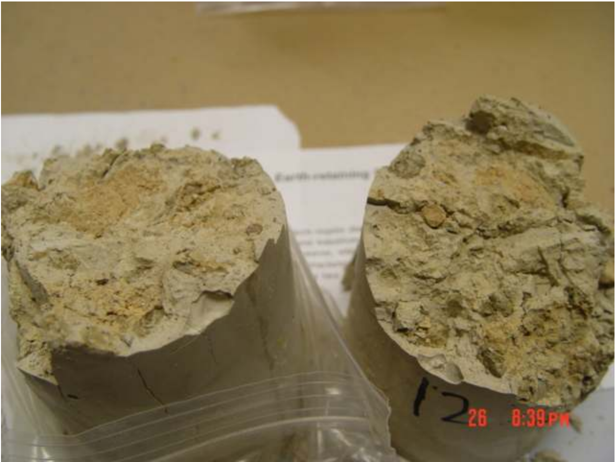
FigureA.5 Cores of Shotcrete Material
