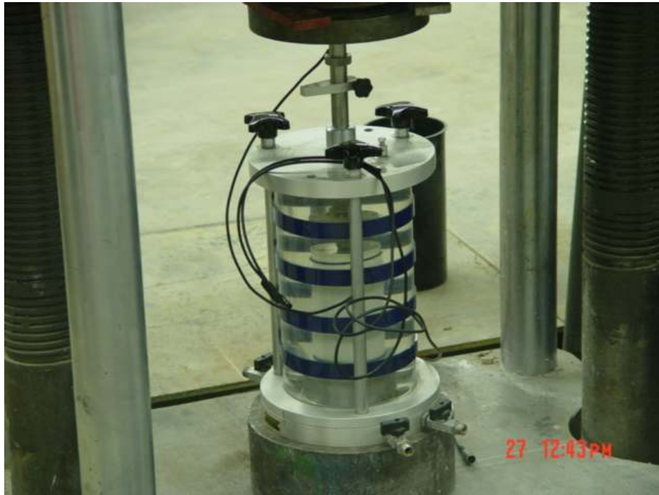
Figure 4.8 Loading of Specimen in 400 kip Tensile Compression Machine
