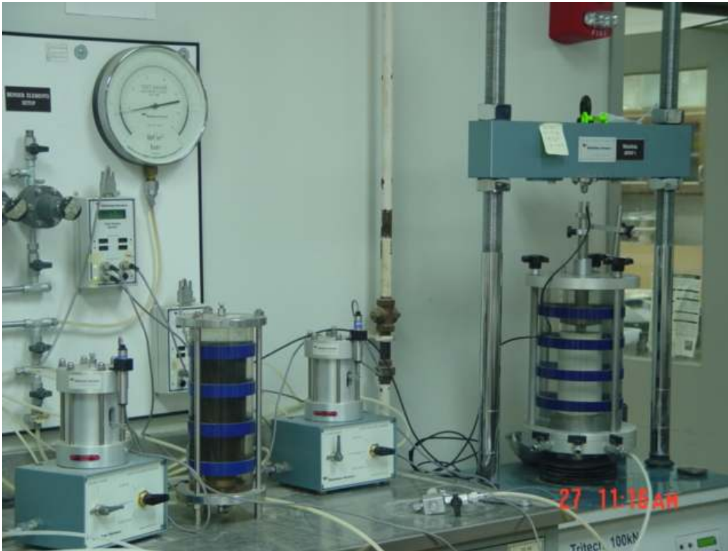
Figure 4.7 Initial Application of Confinement in UU Triaxial
