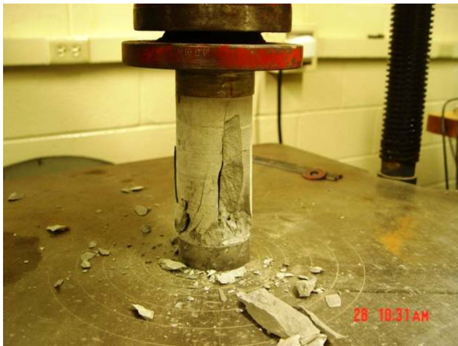
Figure 4.4 Sample Loaded to Failure in UCS Test
