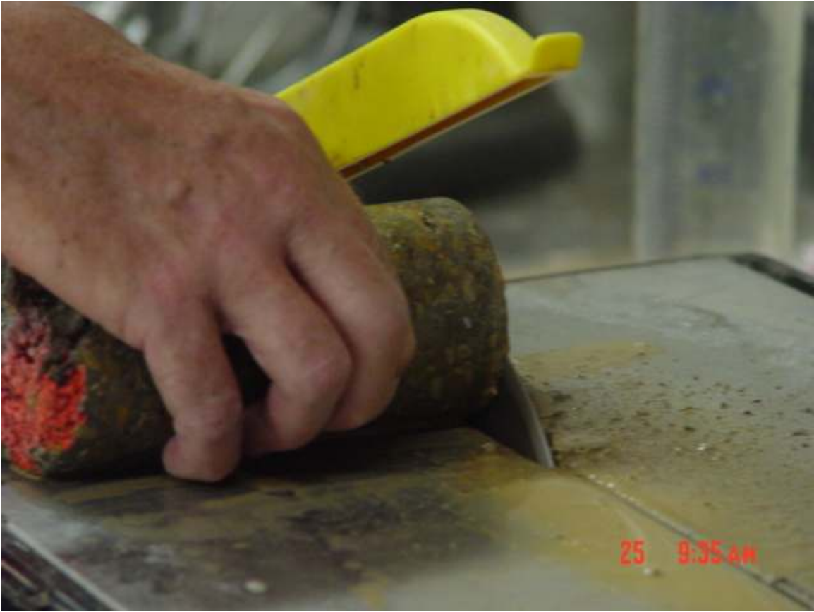
Figure A.1. Preparation of Sample for Engineering Tests
