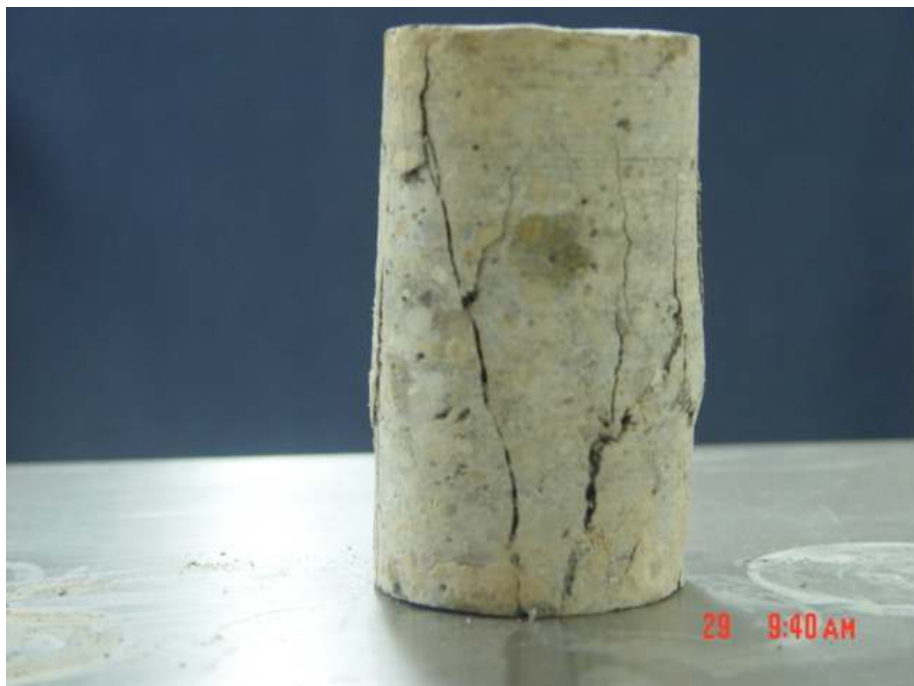
Figure 4.9 UU Triaxial Specimen Loaded to Failure
