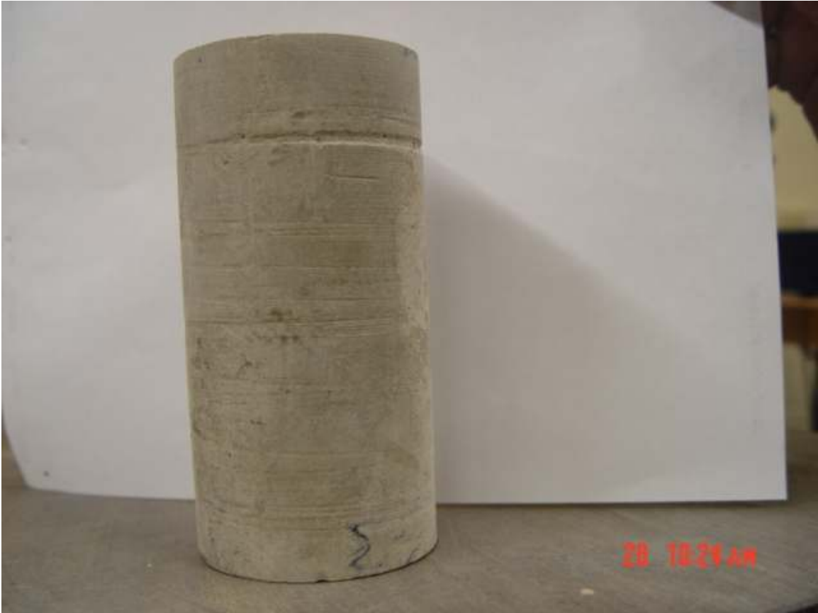
Figure A.4. Representative Specimen for Austin Chalk from DART NC1 _ B Tunnel
