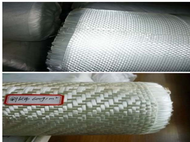
Figure 2.2 Cut FRP Fabric (Source: Verhulst et al, 2001)
