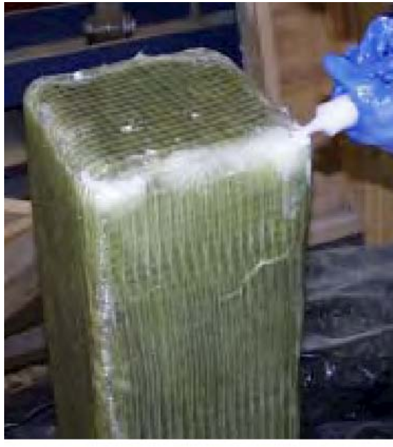
Figure 2.5 Sealing Voids (Source: Verhulst et al, 2001)
