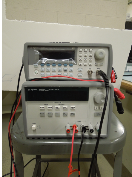
Figure 2.12. Function generator and DC power supply.
