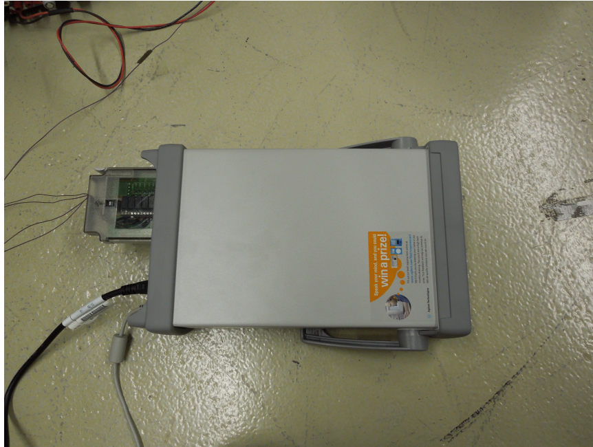
Figure 2.7. Agilent Data Logger with Multiplexer.
