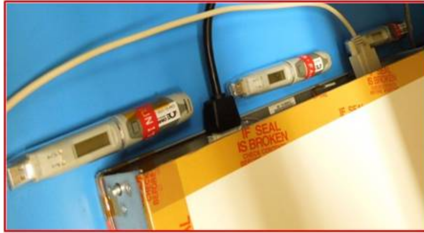
Figure 2.6. Omega USB loggers placed in front of the servers.
