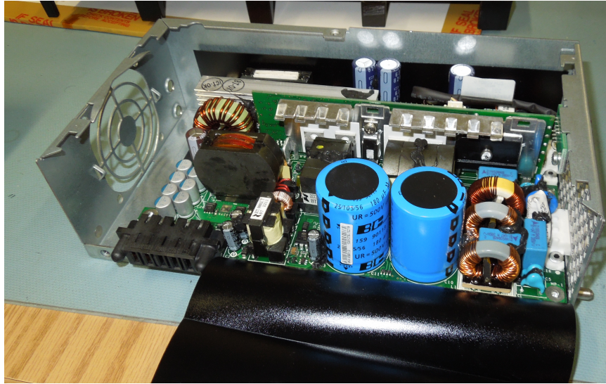
Figure 1.7. Power Supply Unit.
