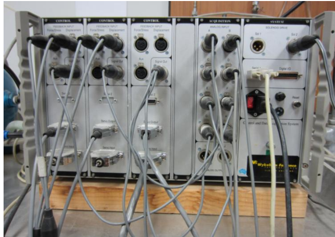
Figure 3.13 The control and data acquisition system
