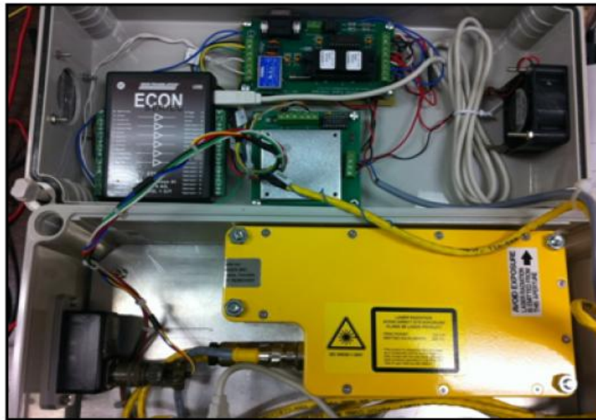
Fig 2.3 Road Profiler Module with Roline Laser[11]
