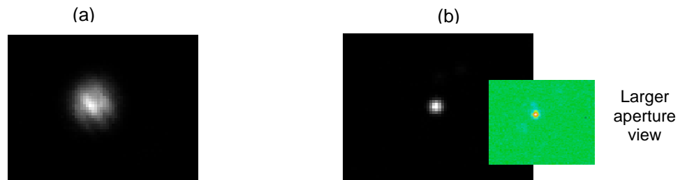
Figure 2.17. (a) Near field image of the green laser beam. (b) Near field fluorescence of quantum dot.
