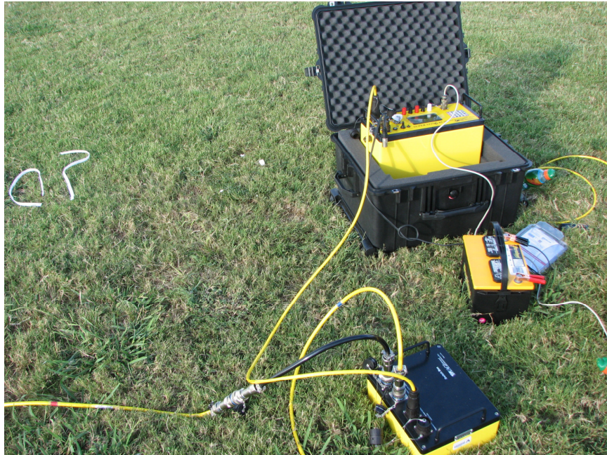
Figure 3.9: SuperSting/Switch box connection
